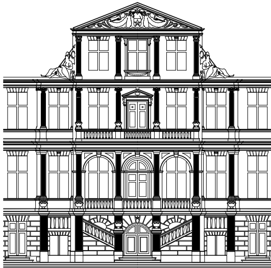
4. Stadhuis decrease in column diameter according to height and less forces to cope with
