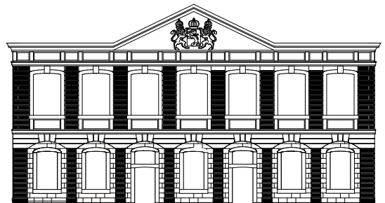
5. Hoofdwacht atectonic increase of 'column' width according to height contradicting the amount of forces to cope with
