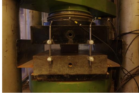
Figure 1 – Compressive test on a single brick.
