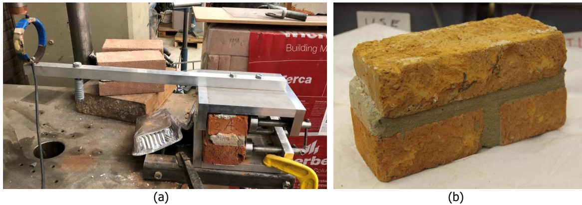
Figure 29 – Bond wrench tests: (a) improved set-up; (b) sawn-cut couplet specimens.
