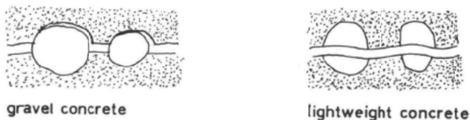
Fig. 3.33: Aggregate interlock in gravel concrete (intermediate or low strength) and lightweight concrete. (Walraven, 1980).
