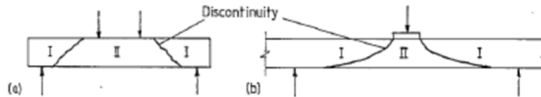
Fig. 3.157: Discontinuities in shear failures (Cope and Clark, 1984).
