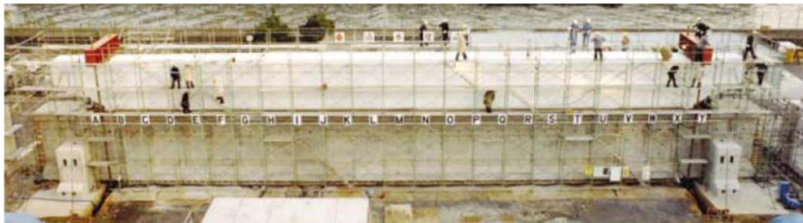
Fig. 3.63: Large beam failing in shear (Lubell et al., 2004).
