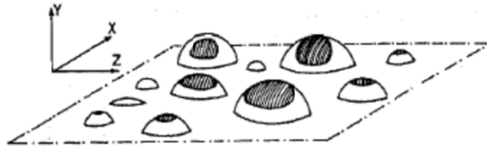
Fig. 3.37: Contact areas during sliding (Walraven, 1981).
