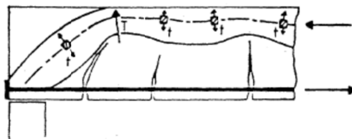
Fig. 3.27: Schematic representation of region of compressive force path (Kotsovos, 1992).
