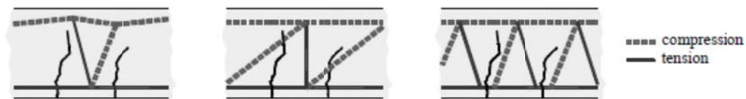
Fig. 3.25: Mechanism of shear transfer without shear reinforcement: cantilever action, aggregate interlock and dowel action (Muttoni and Schwartz, 1991).
