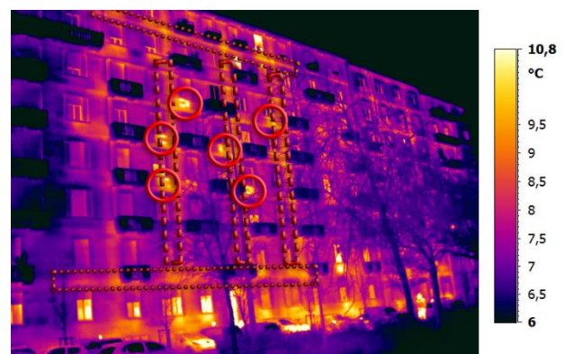
Figure 5 – Thermogram of the eastern façade of Case Study 2; outdoor air temperature 8 C, emissivity 0.92.
