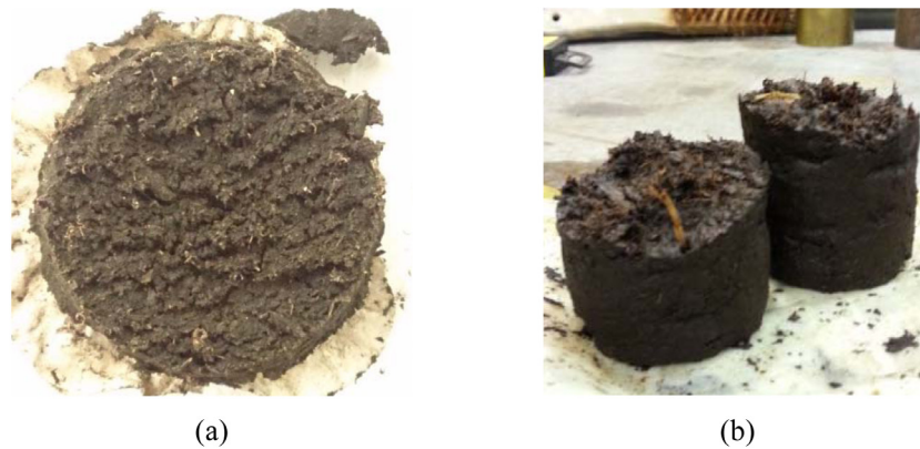
Fig. 19. Reconstituted peat sample (a), and (b) natural peat sample with the twisted and warped big fibres visible in the peat matrix.
