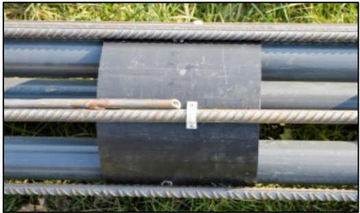
Figure 2: Structural adjustment to create flaws. Protection ring and injection tube for bulge.
