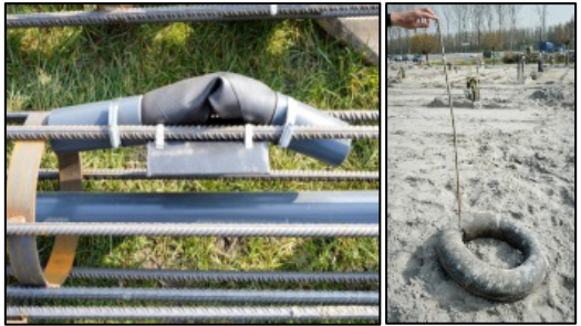
Figure 3: Structural adjustment to create flaws. Rubber tire and a filled injection tube for neck (bottom right). Top: symmetric neck. Bottom left: asymmetric neck.
