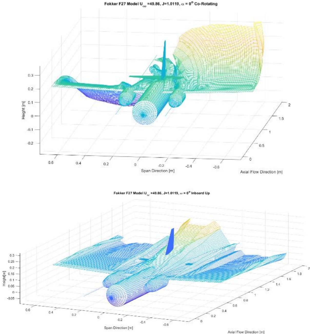
Figure 68: The Excessive Rolling by the Co-Rotating Propeller in the Vortex Flow Field
