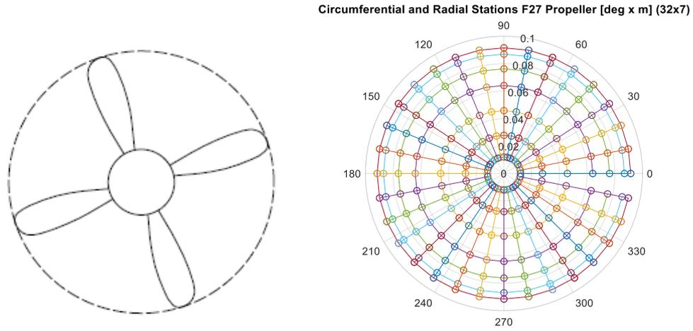
Figure 50: F27 Propeller Divided into Stations of Discrete Points
