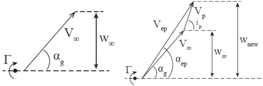
Figure 20: Velocity Diagram for a Single Wing (Left) and Wing+Propeller (Right) [33]
