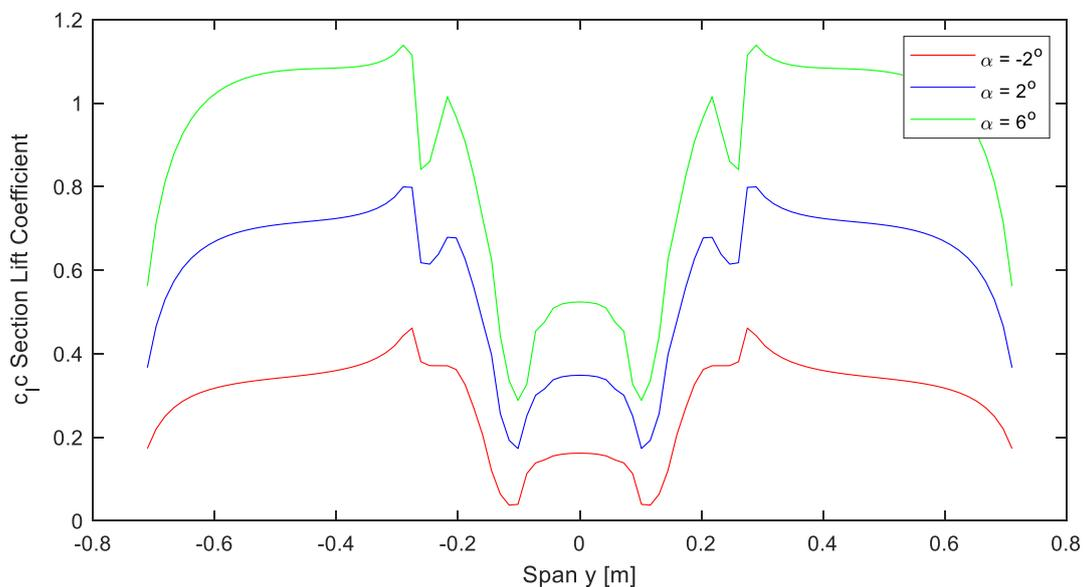
Figure 80: Section Lift Distribution along the F27 Wing Span  $U_\infty = 50 \text{ m/s}$ ,  $Re = 0.41 \cdot 10^6$ ,  $M = 0.145$ ,  $J = 0.801$ , OU
