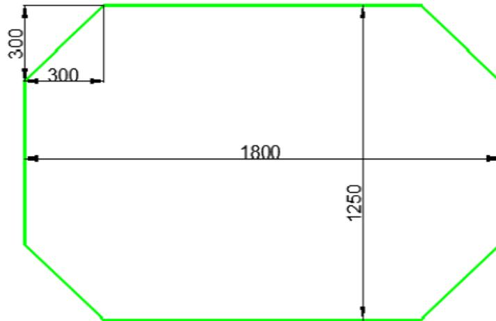
The contraction ratio of the wind tunnel is 1:17.8 and maximum turbulence is around 0.07%.
