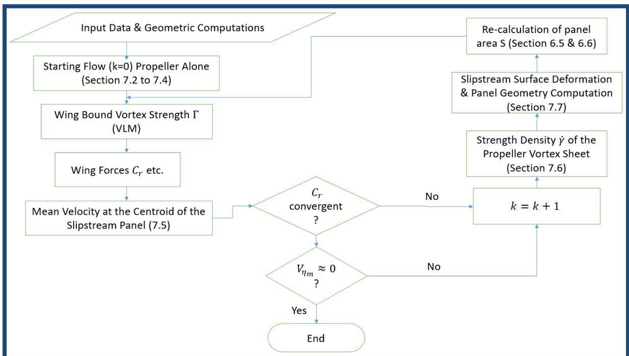
Figure 44: Flowchart for the SVPM Case with Slipstream Deformation
