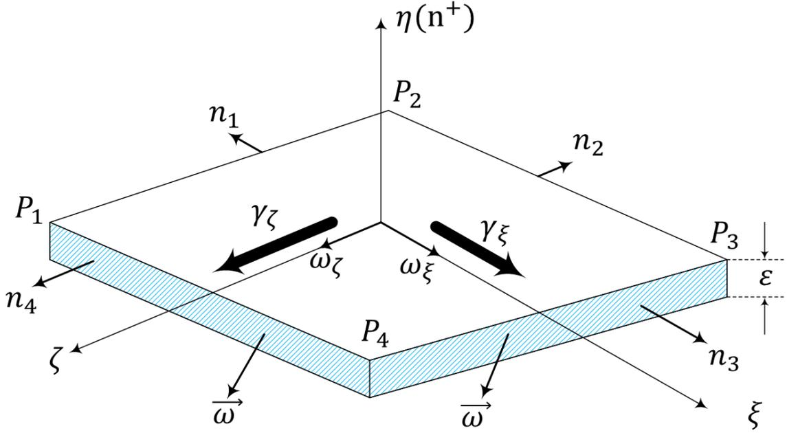
Figure 36: Vorticity Flux on a Panel Element [15]
