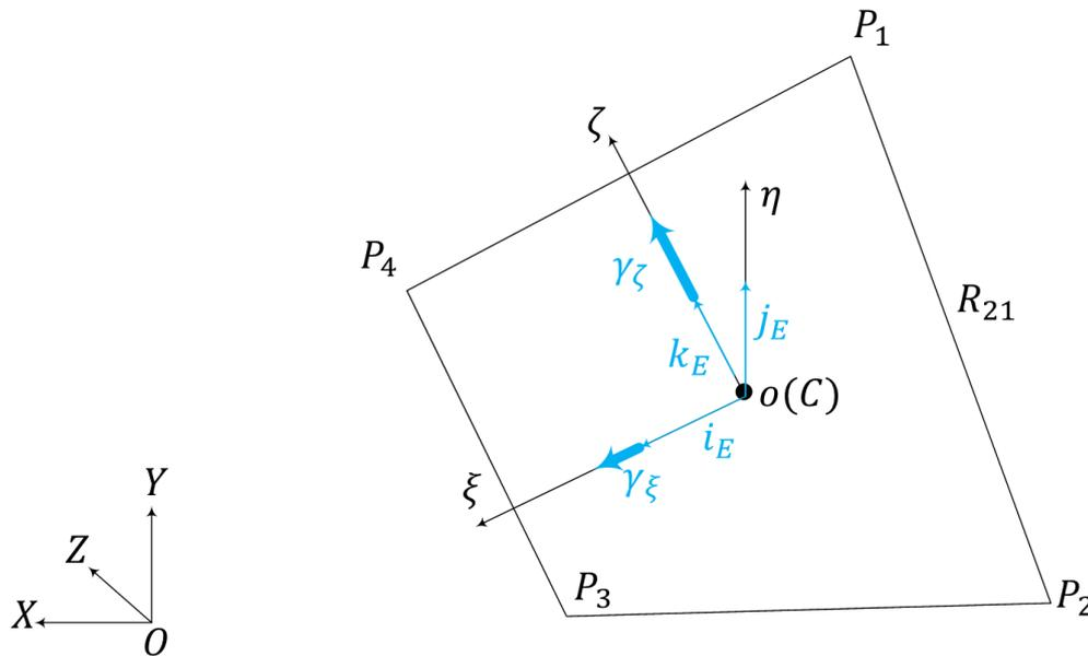
Figure 29: Local Coordinate System for a Panel [15]
