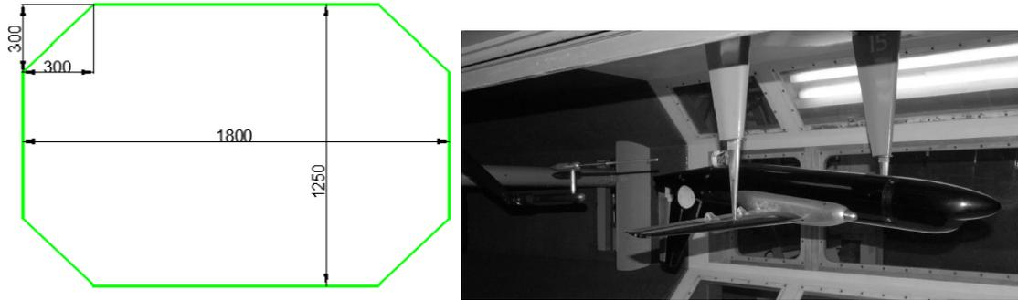
Figure 64: Test Cross-Section of the Wind Tunnel (Left) and Fokker F27 Installed in the Test Section (Right) [34]
