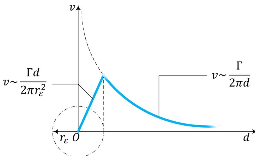
Figure 33: Induced Velocity by Rankine Vortex with Varying Distance [15]
