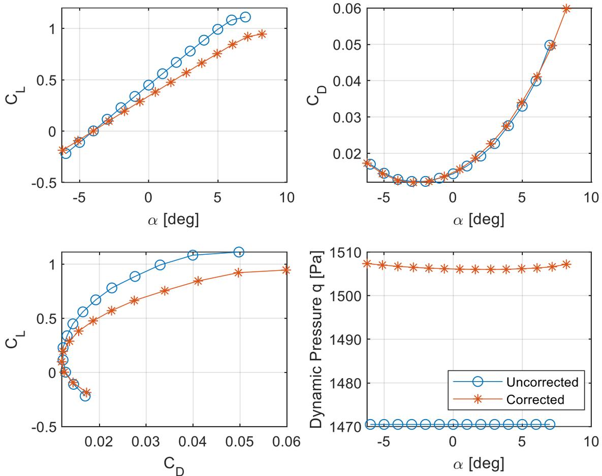
Figure 75: WFNVHP Aerodynamic Parameters at 270 rps,  $U_\infty = 50 \text{ m/s}$ ,  $Re = 0.41 \cdot 10^6$ ,  $M = 0.145$
