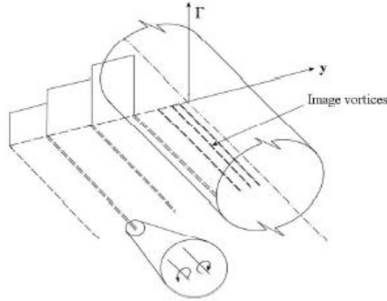
Figure 59: Horseshoe Vortices and Their Image in the Fuselage [63]
