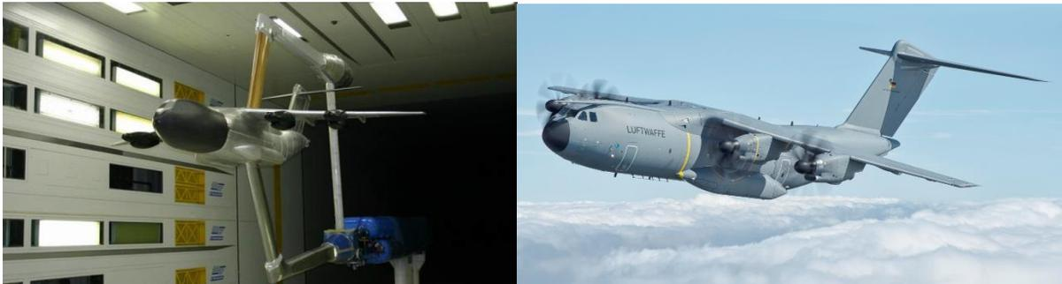
Figure 17: AIRBUS A400M Model in Wind Tunnel (Left) [27]
