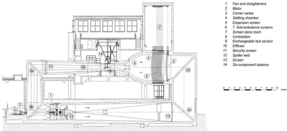
It is a closed return wind tunnel with a maximum achievable speed of approximately 120 m/s. It is driven by a 525 kW DC motor and is built on two floors. The maximum Reynolds number achievable is around  $3.5 \cdot 10^6$ . The test section area is given below:
