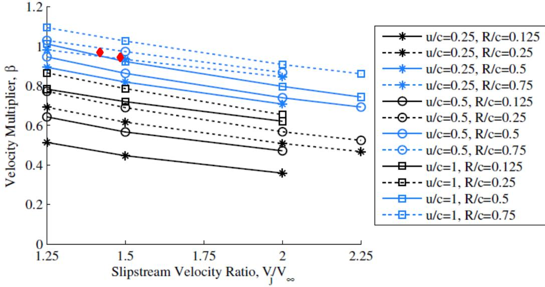
Figure 90:  $\beta$  Values for Various Propeller/Wing Configurations [50] (Red Dots are the Corresponding Points to the Experiment)
