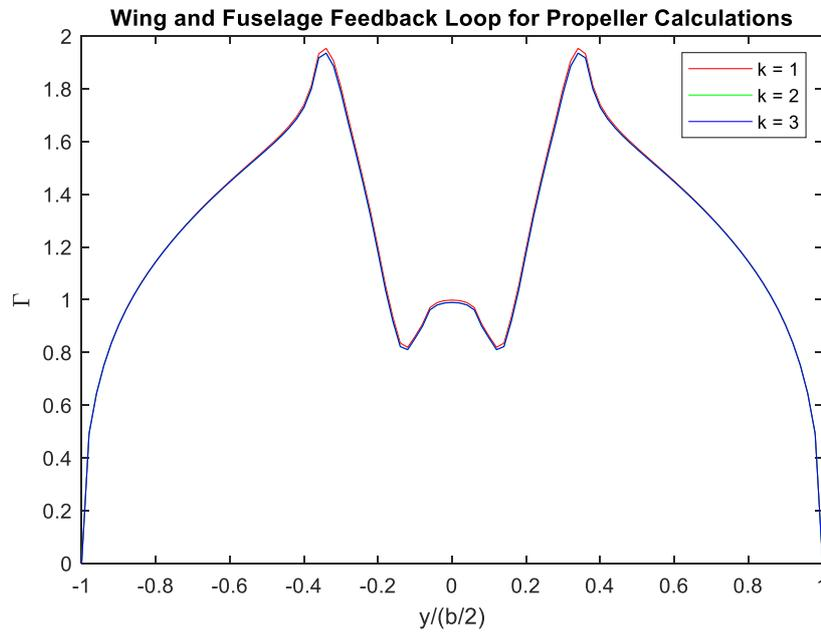
Figure 66: Spanwise Circulation for  $k$  Number of Iterations
