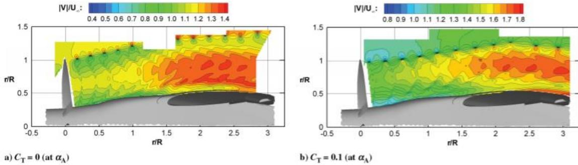
Figure 14: Magnitude of Instantaneous Velocities at the Slipstream for Different Thrust Cases [42]
