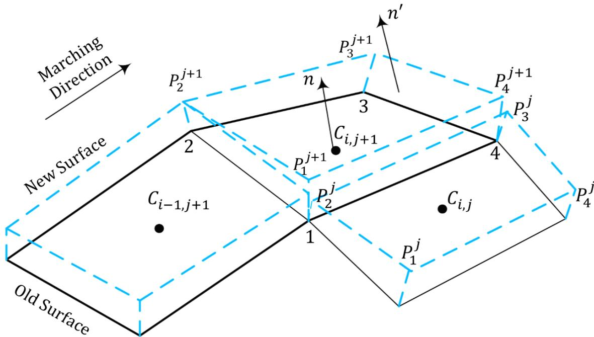
Figure 38: Deformed Slipstream Panel [15]
