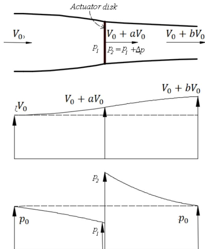
Figure 100: Velocity Increase and Pressure Jump along the Slipstream in ADM [46]
