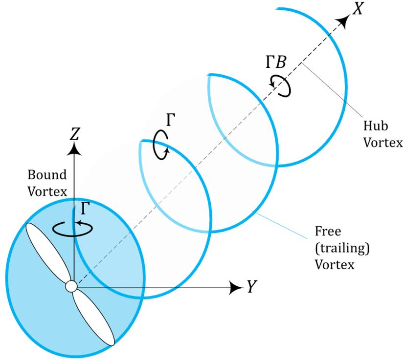
Figure 32: Definition of the Vortices in the Slipstream [15]
