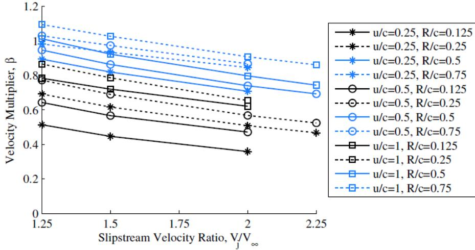
Figure 22:  $\beta$  Values for Various Propeller/Wing Configurations [50]
