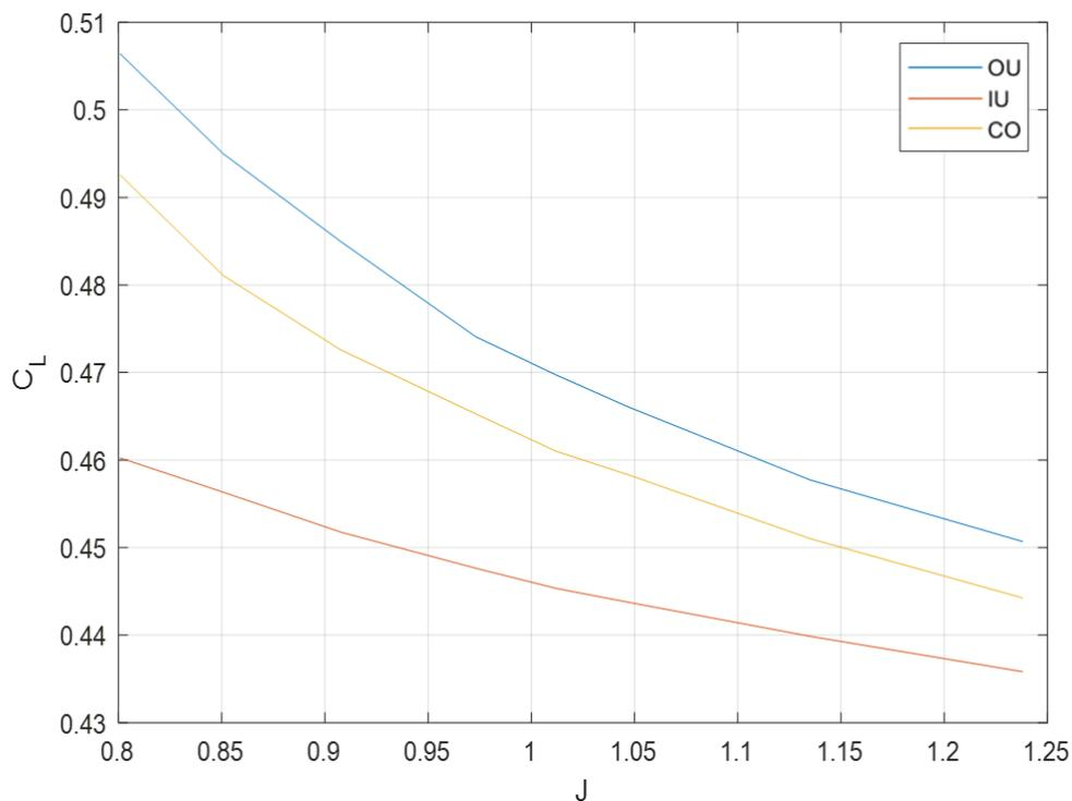
Figure 88: F27 Panel Method  $C_L$  vs.  $J$ ,  $U_\infty = 50$  m/s,  $Re = 0.41 \cdot 10^6$ ,  $M = 0.145$
