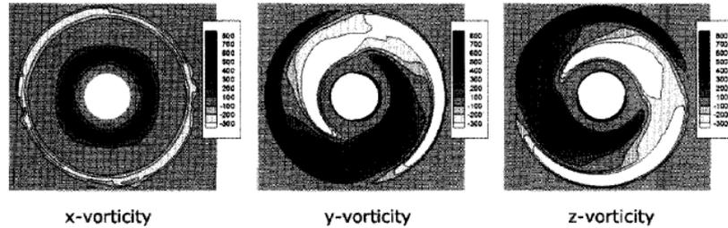
Figure 103: Visualization of The Vorticity Vectors Behind the Propeller [70]
