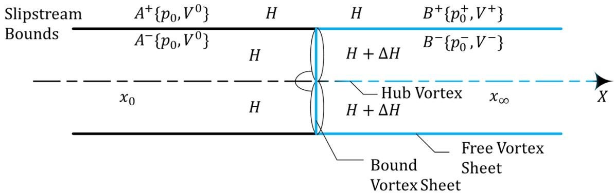
Figure 35: Different Pressures Inside and Outside Slipstream Boundary [15]
