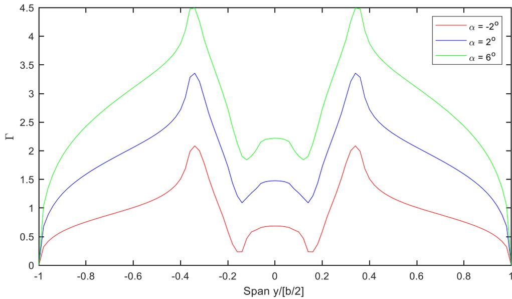
Figure 79: Circulation Distribution along the F27 Wing Span,  $U_\infty = 50 \text{ m/s}$ ,  $Re = 0.41 \cdot 10^6$ ,  $M = 0.145$ ,  $J = 0.801$ , OU
