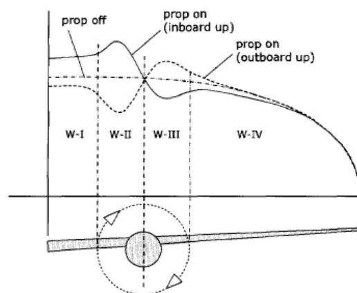
Figure 9: Lift Distribution under Propeller Slipstream [4]
