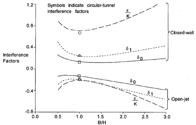
Figure 109: Change in Lift Interference Factor  $\delta$  with Varying Breadth-to-Height Ratio ( $B/H$ ) AGARD 109 (Left) AGARD 336 (Right)
