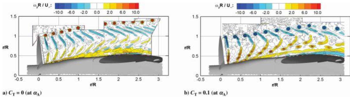
Figure 15: Vorticity Profile at the Slipstream for Different Thrust Cases [42]
