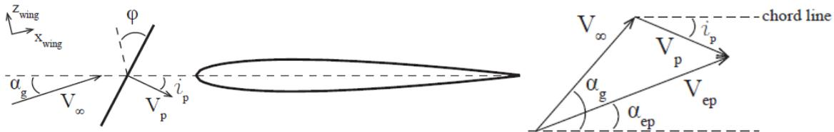
Figure 19: Diagram of the Propeller Incoming Flow in 2D Wing Airfoil Section [33]
