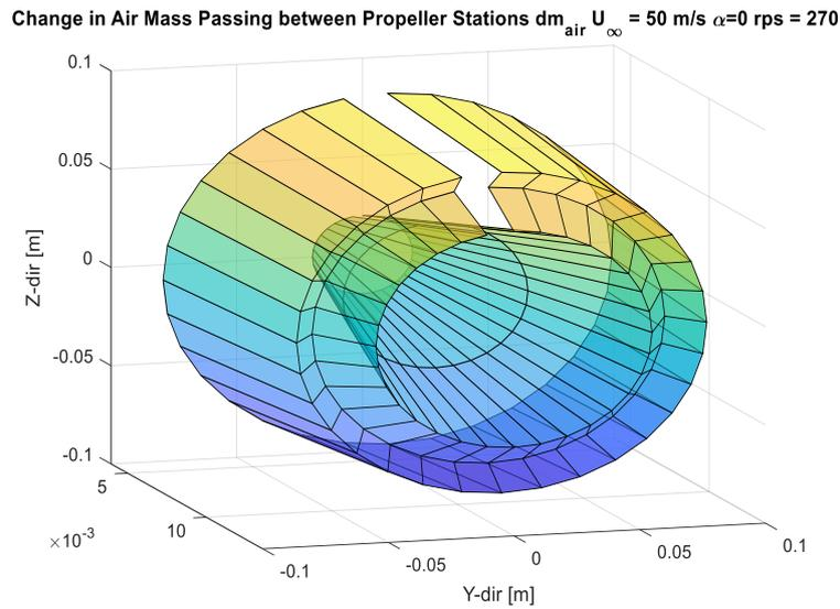
Figure 56: 3D Visualization Air Mass Passing between Propeller Stations  $dm_{air}$  [kg]
