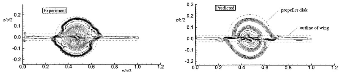
Figure 46: Slipstream Shearing Observed by Veldhuis in PROWIM [4]
