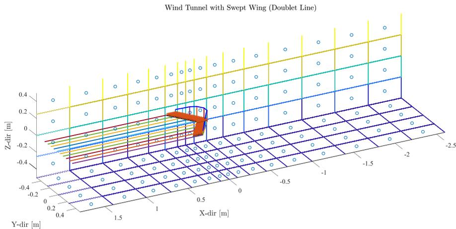
Figure 106: Cross-Section of the Wind Tunnel Panel Code
