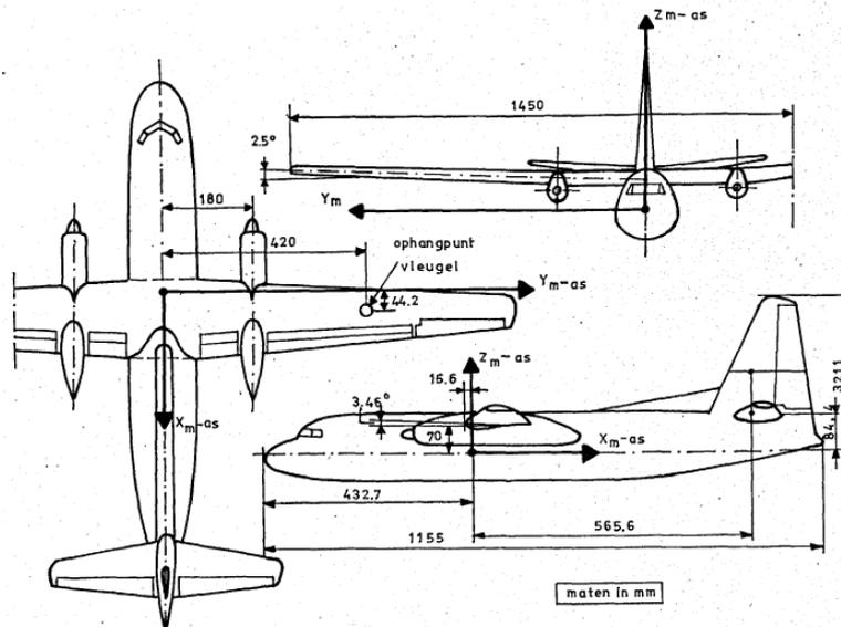
Figure 23: Dimensions of Fokker F27 1:20 Scale Model [54]
