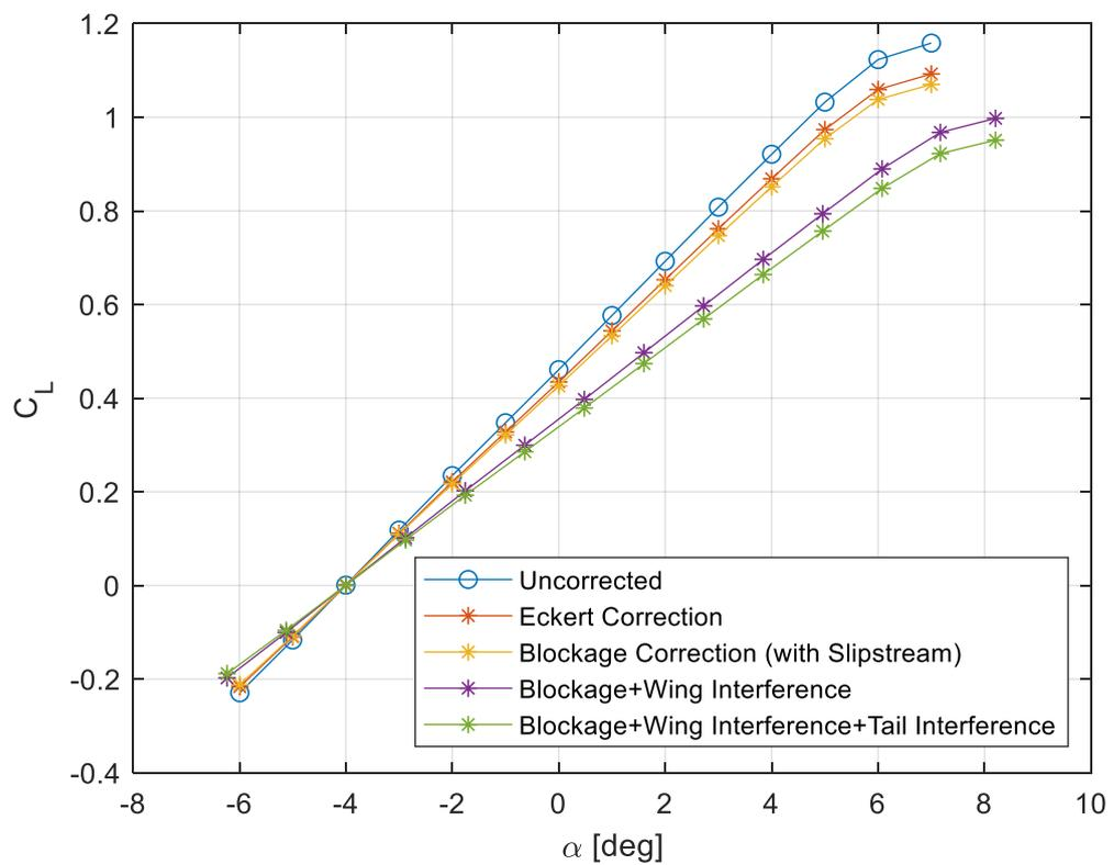
Figure 77: Visualized Impact of Correction Methods including Eckert  $rps = 320$  (Down),  $rps = 270$  (Up),  $U_\infty = 50 \text{ m/s}$ ,  $Re = 0.41 \cdot 10^6$ ,  $M = 0.145$
