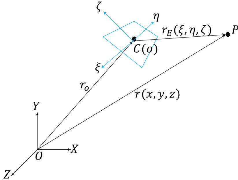
Figure 30: Distance from Local and Global Reference Points [15]
