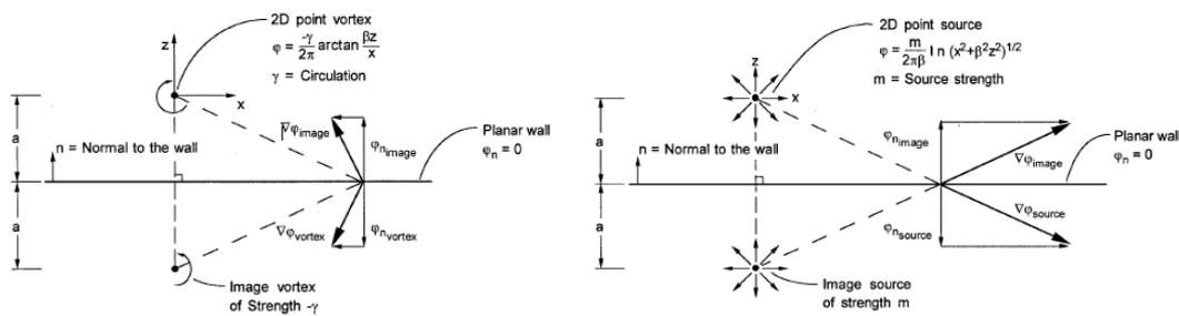
Figure 5: Mirror Images on 2D Plane for a Vortex (Left) and for a Source (right) [31]
