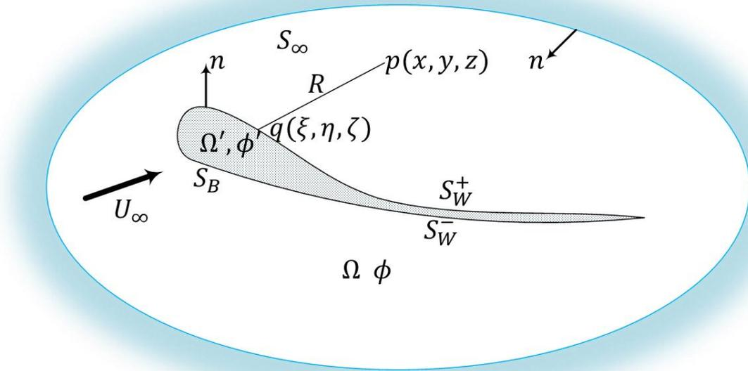
Figure 25: Notations Used in A General Body with Closed Domain [22]
