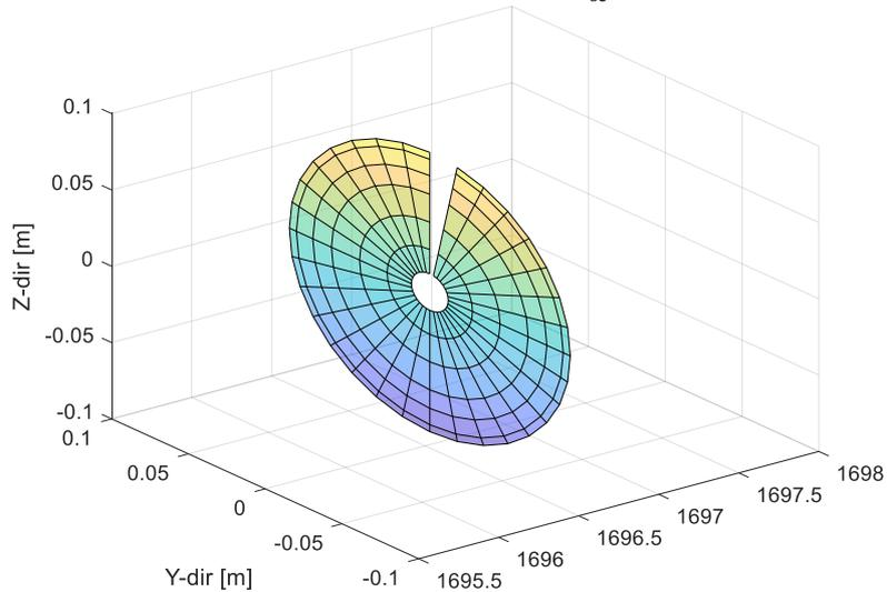
**Figure 53: 3D Visualization of Angular Velocity at the Propeller Plane  $\omega$  [rad/s]**
