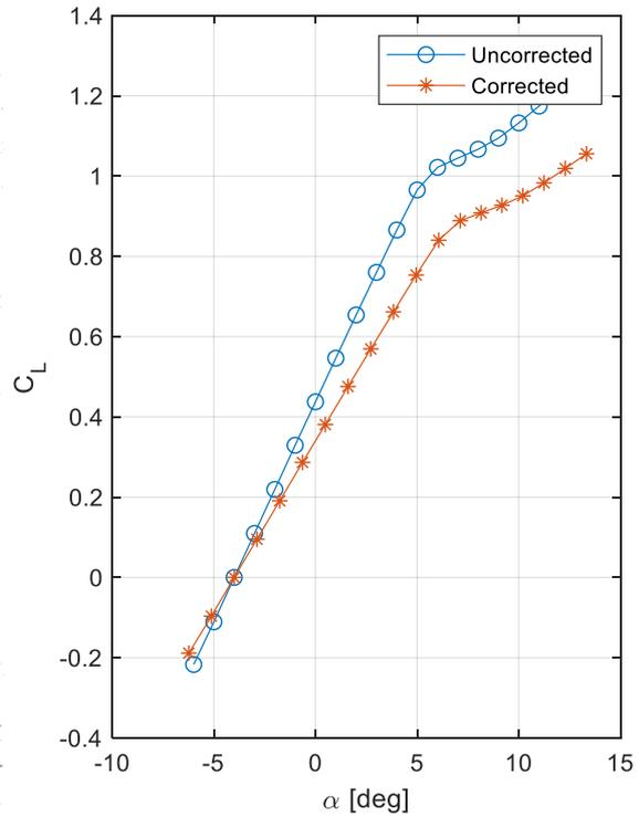
Figure 73: F27  $C_L$  vs.  $\alpha$ , Binkhorst's Lift Curve at  $U_\infty \approx 85$  m/s,  $Re = 0.7 \cdot 10^6$ ,  $M = 0.247$  (Left), *WFNVH* at  $U_\infty = 80$  m/s,  $Re = 0.66 \cdot 10^6$ ,  $M = 0.232$  (Right) [54]
