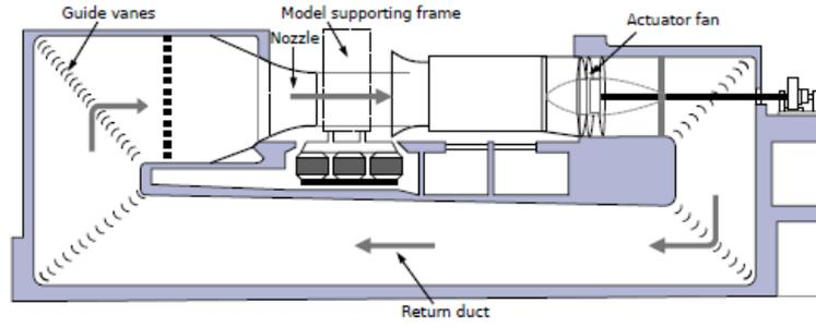
Figure 4: Closed Return Wind Tunnel Plan [34]
