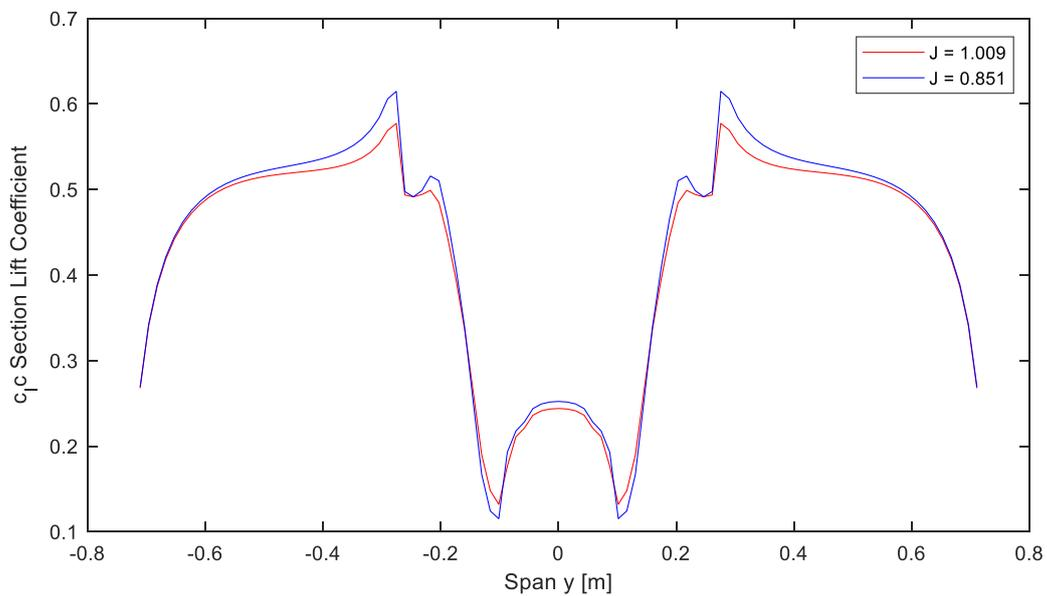
Figure 84: Section Lift Distribution along the F27 Wing Span  $U_\infty = 50 \text{ m/s}$ ,  $Re = 0.41 \cdot 10^6$ ,  $M = 0.145$ ,  $\alpha = 0^\circ$ , OU
