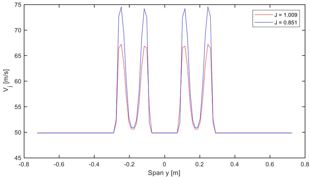
Figure 89: Jet Velocity  $V_j$  [m/s] Along the F27 Wing (Peak Velocity is Used for Patterson)
