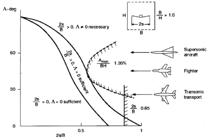
Figure 105: Modelling Requirements for Wings [73]
