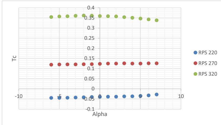
Figure 65: Uncorrected  $T_c$  vs.  $\alpha$  at Three Different  $rps$  Values,  $Re = 0.41 \cdot 10^6$
