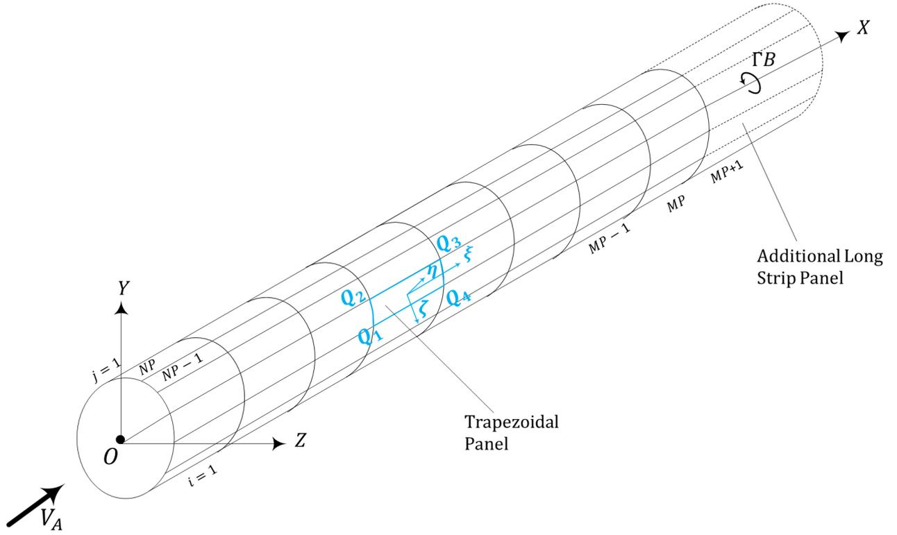
Figure 31: Slipstream Panel Representation with Mapping [15]
