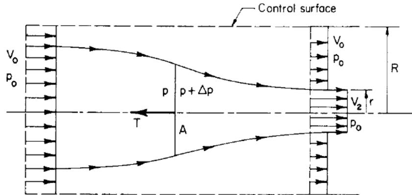
Figure 99: Streamtube and Control Surface for the Actuator Disk [57]
