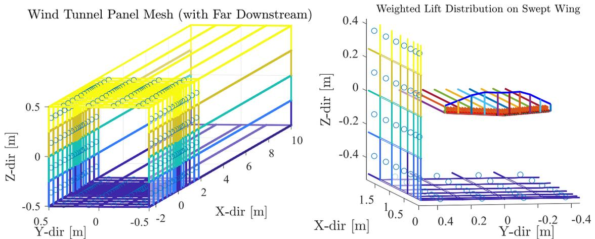
Figure 107: Layout of the Panels based on Keller's Parameters (Left), Visualized Swept Wing Lift Distribution (Right)
