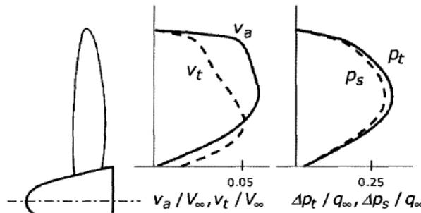
Figure 102: Axial and Tangential Velocity and Pressure Distribution on the Propeller [4]
