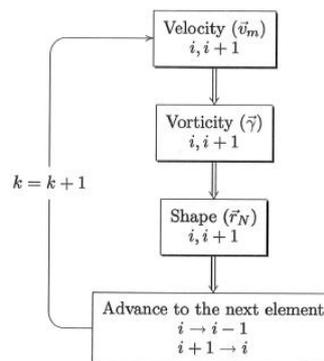
Figure 48: New Iteration Scheme for the Vorticity Panel Method [56]
