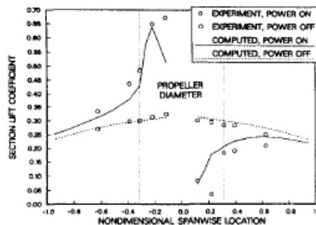
Fig. 5. Computed and Experimental Lift Distribution for Power on Conditions. ( $J = 2.0$ ,  $\alpha = 0$  degrees,  $Mach = 0.5$ ).
