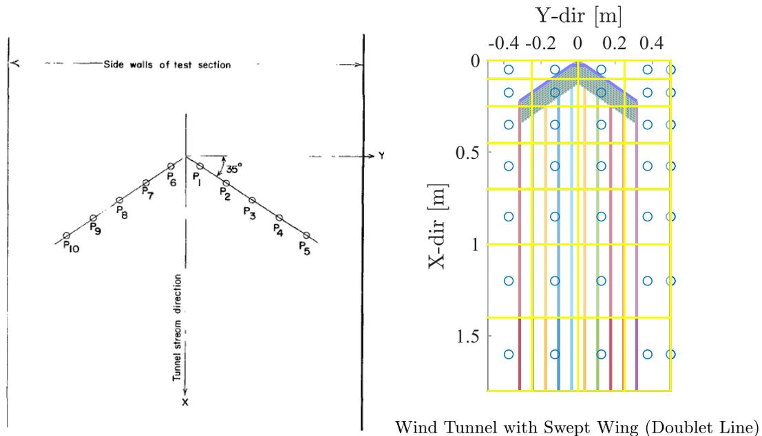
Figure 108: Swept Wing Used by Keller (from Wright) [77] (Left) and Swept Wing with Doublet Lines in Panel Code (Right)
