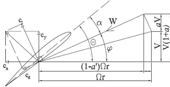
Figure 49: Blade Element Diagram with Relative Induced Velocities [62]
