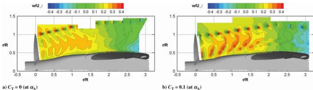
Figure 16: Vertical Velocity Component at the Slipstream for Different Thrust Cases [42]
