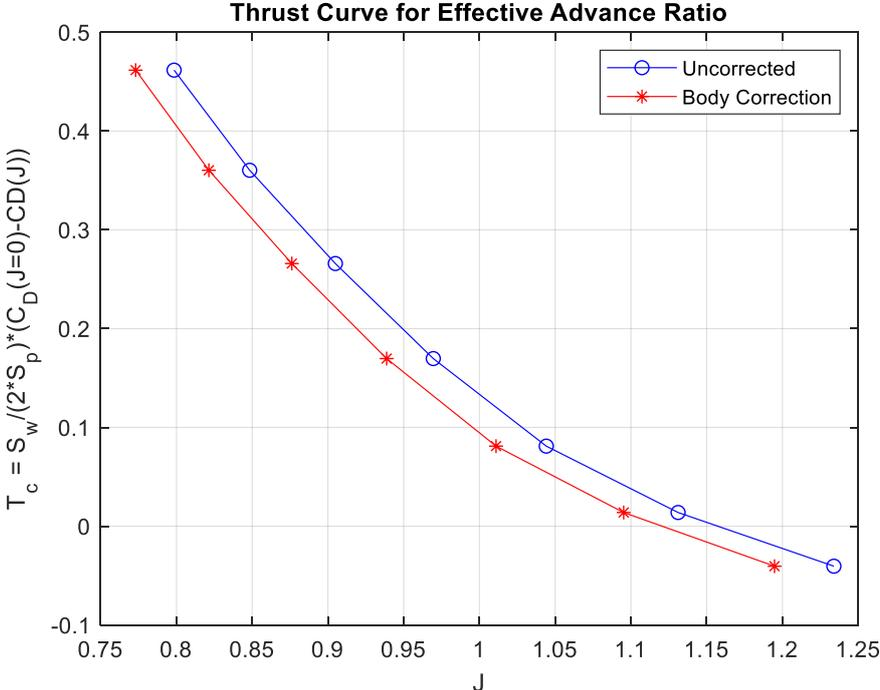
Figure 78: Body Correction  $J_E$  for RPS Sweep,  $U_\infty = 50 \text{ m/s}$ ,  $Re = 0.41 \cdot 10^6$ ,  $M = 0.145$
