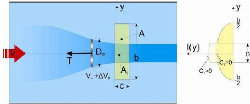
Figure 18: Single Propeller Effect on the Lift Distribution according to Eckert Method [27]
