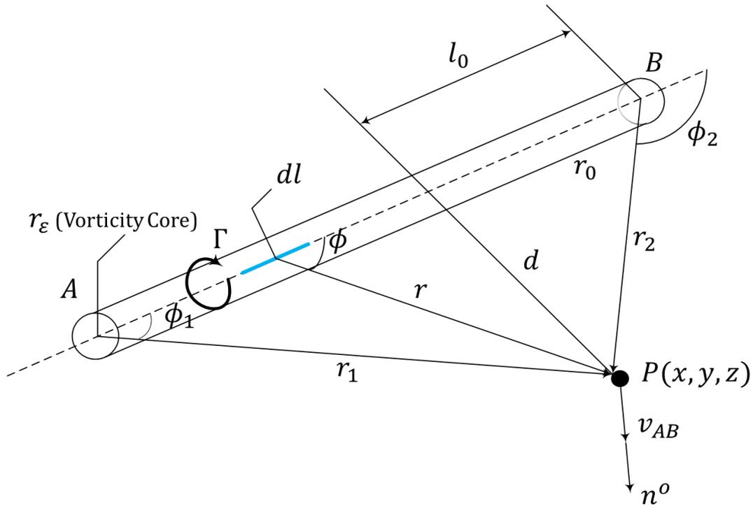
Figure 34: Vortex Filament Geometry [15]
