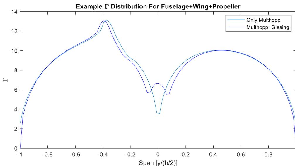
Figure 61: Gamma Distribution along the Wing Chord with Fuselage Effects
