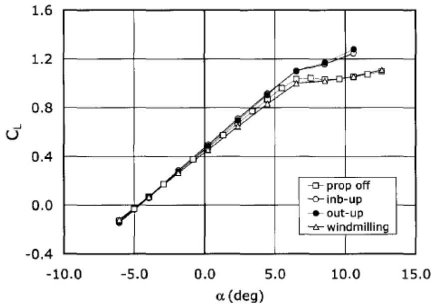
Figure 85: F27 Propeller Installed Wind Tunnel  $C_l$  vs.  $\alpha$ ,  $U_\infty \approx 50$  m/s,  $Re = 0.41 \cdot 10^6$  [4]
