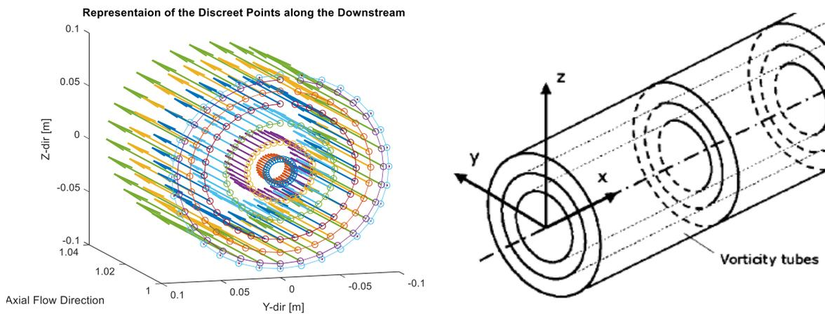
Figure 51: Representation of F27 Propeller Along Downstream (Left) and Vorticity Tube Representation (Right) [4]
