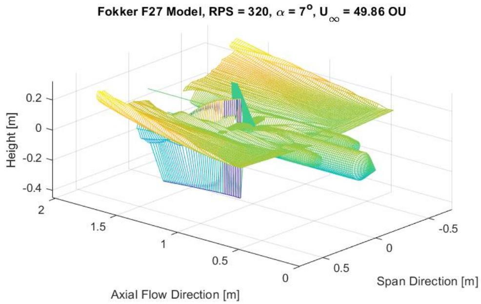
Figure 70: Excessive Panel Deformation at the Starboard Side Horizontal Tail Root
