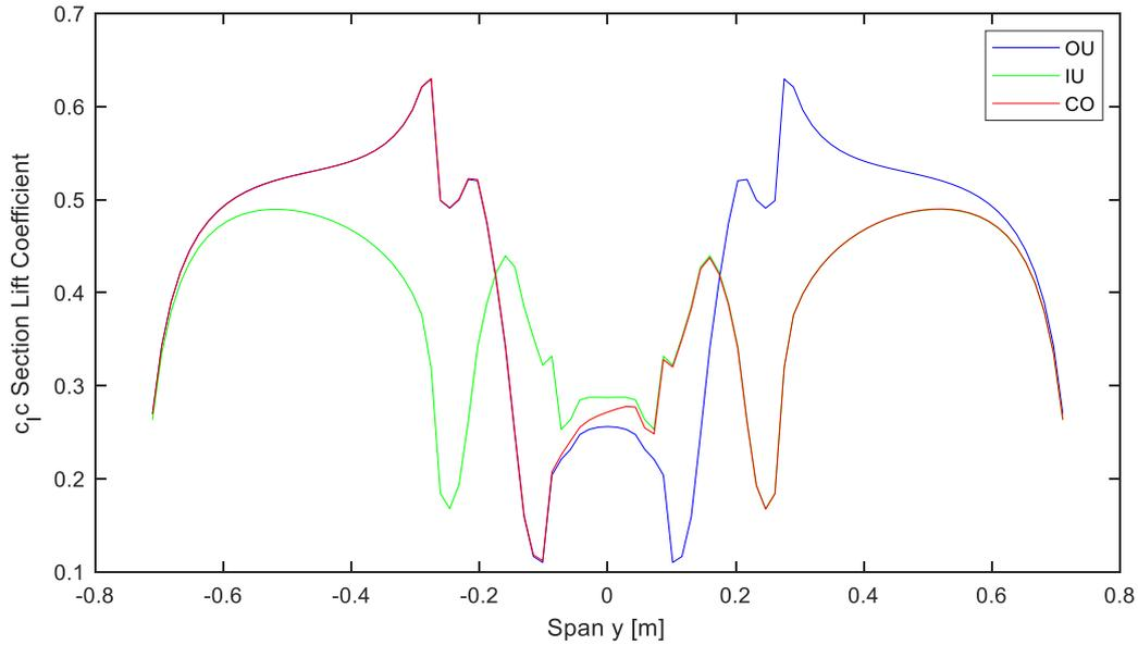
Figure 82: Section Lift Distribution along the F27 Wing Span  $U_\infty = 50 \text{ m/s}$ ,  $Re = 0.41 \cdot 10^6$ ,  $M = 0.145$ ,  $J = 0.801$ ,  $\alpha = 0^\circ$
