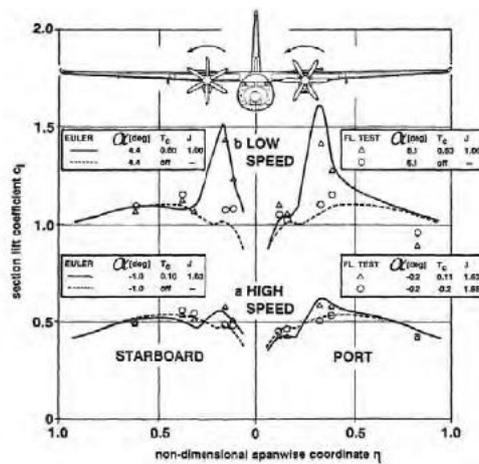
Figure 10: The Experimental and Computed Section Lift Distribution for Fokker 50 [12]
