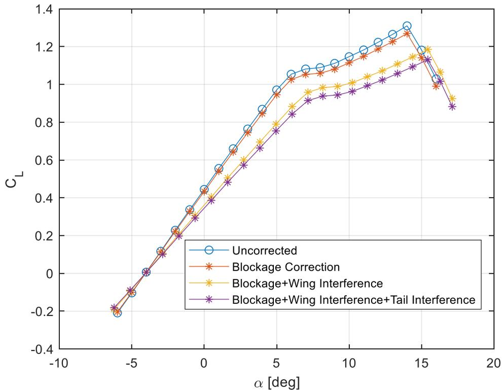
Figure 72: Visualized Impact of Each Correction Method, *WFNVH* at  $U_\infty = 50 \text{ m/s}$ ,  $Re = 0.41 \cdot 10^6$ ,  $M = 0.145$
