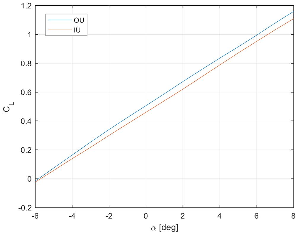
Figure 86: F27 Panel Method  $C_L$  vs.  $\alpha$ ,  $U_\infty = 50 \text{ m/s}$ ,  $Re = 0.41 \cdot 10^6$ ,  $M = 0.145$ ,  $J \approx 0.81$
