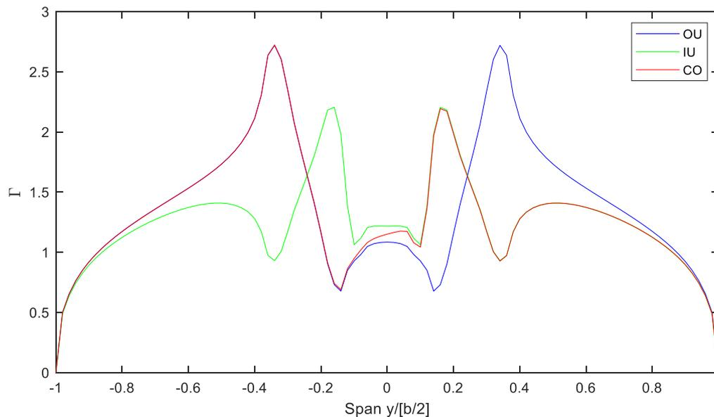
Figure 81: Circulation Distribution along the F27 Wing Span,  $U_\infty = 50 \text{ m/s}$ ,  $Re = 0.41 \cdot 10^6$ ,  $M = 0.145$ ,  $J = 0.801$ ,  $\alpha = 0^\circ$
