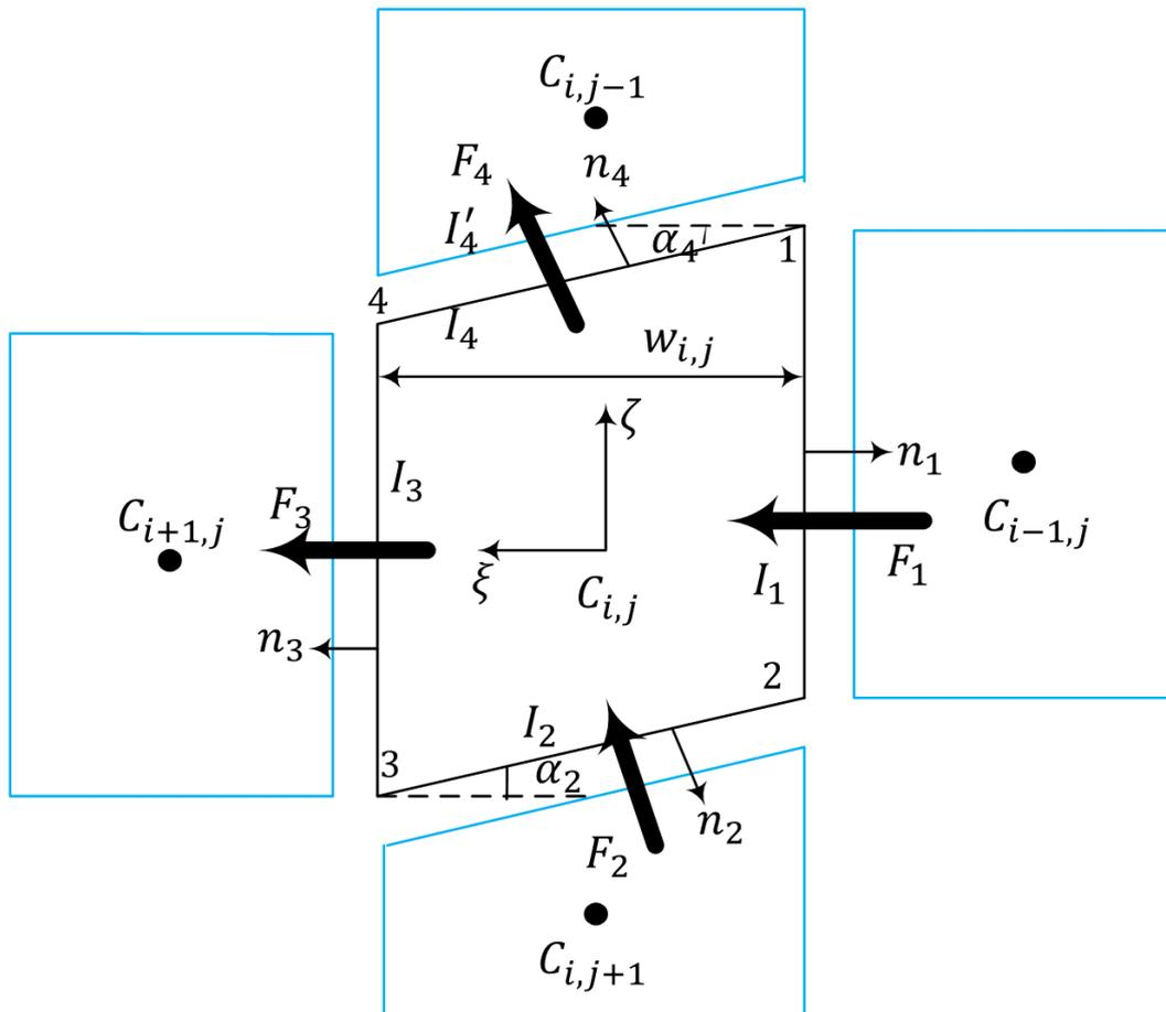
Figure 37: Panel Notation on a Control Volume with Vorticity Fluxes [15]
