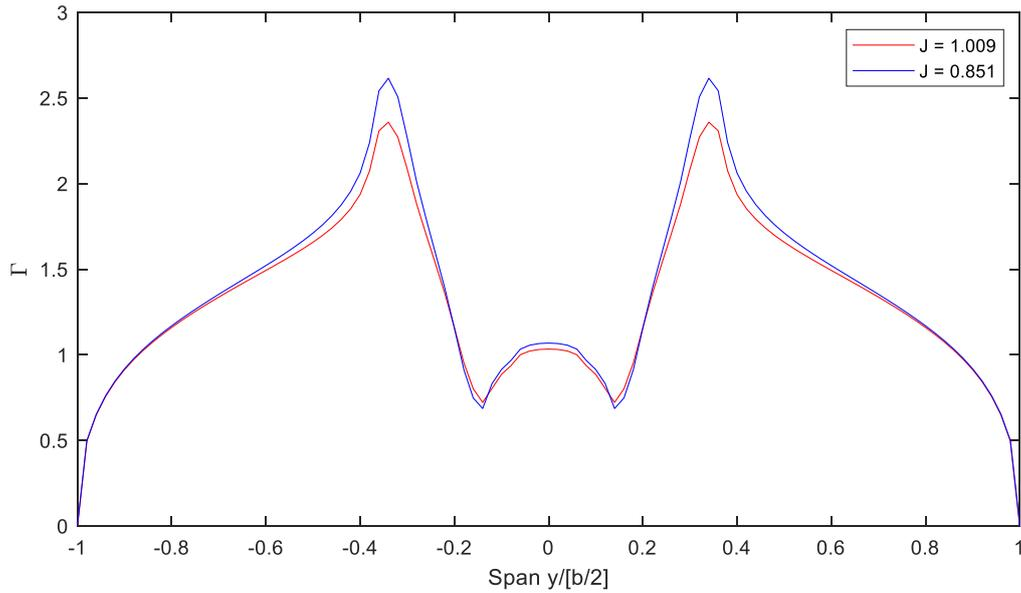
Figure 83: Circulation Distribution along the F27 Wing Span,  $U_\infty = 50 \text{ m/s}$ ,  $Re = 0.41 \cdot 10^6$ ,  $M = 0.145$ ,  $\alpha = 0^\circ$ , OU
