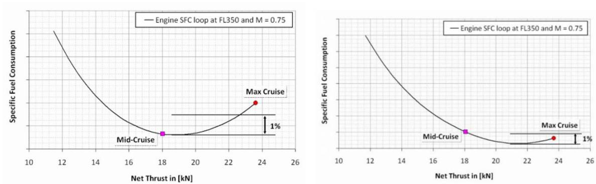
Figure 2: The Operation Range and Corresponding Change of Fuel Consumption for Turbofan (Left) and Turboprop (Right) Propulsion Systems (study made by Volvo Aero) [10]
