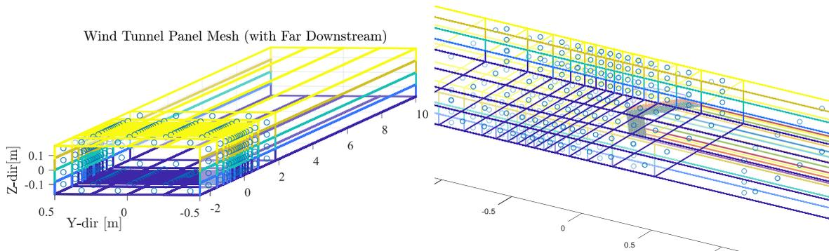
Figure 110: Example of A Wind Tunnel with  $B/H = 3$  (Left) and Swept Wing Placed in a Higher Concentrated Panel Distribution to the Center Point/Wing Tip (Right)
