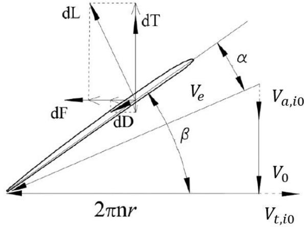
Figure 101: Forces on the Propeller Airfoil Section in BEM [46]
