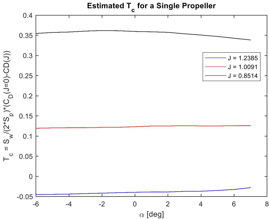
Figure 74: Distribution of Thrust Coefficients at Different  $\alpha$  and Different Advance Ratio  $J$
