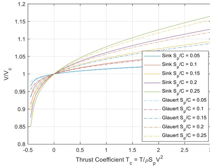
Figure 7: Comparison of Glauert and Sink Method for Slipstream Blockage
