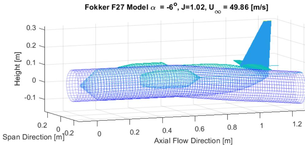
Figure 69: Slipstream Tube Going under the Horizontal tail
