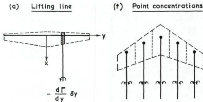
Figure 104: Two Different Ways of Modeling Wing in Potential Flow [26]
