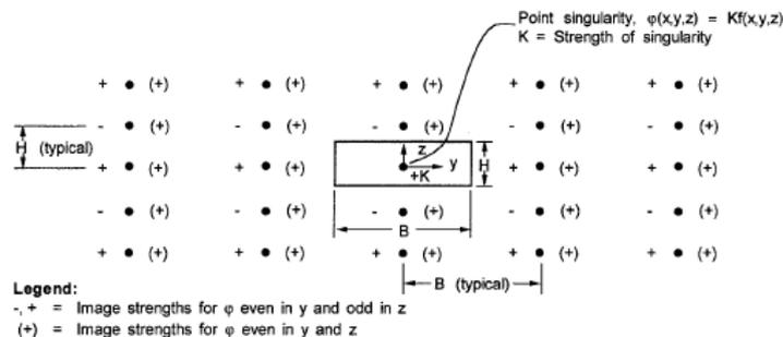
Figure 6: Example of System of Images for a Singularity [31]
