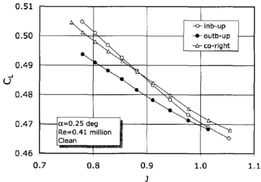
Figure 87: F27 Propeller Installed Wind Tunnel  $C_L$  vs.  $J$ ,  $U_\infty \approx 50 \text{ m/s}$ ,  $Re = 0.41 \cdot 10^6$  [4]
