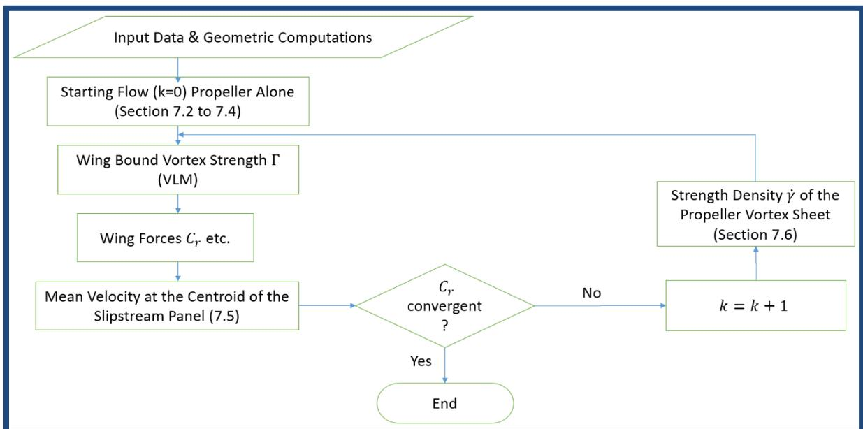
Figure 39: Flowchart Used to Test the SVPM Algorithm
