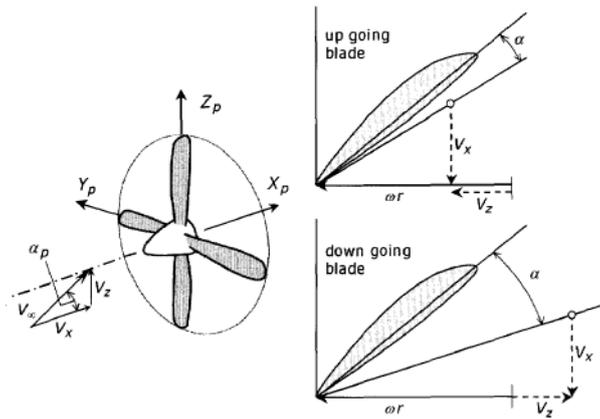
Figure 8: Change in Incoming Flow Angle for Propeller Blades [4]
