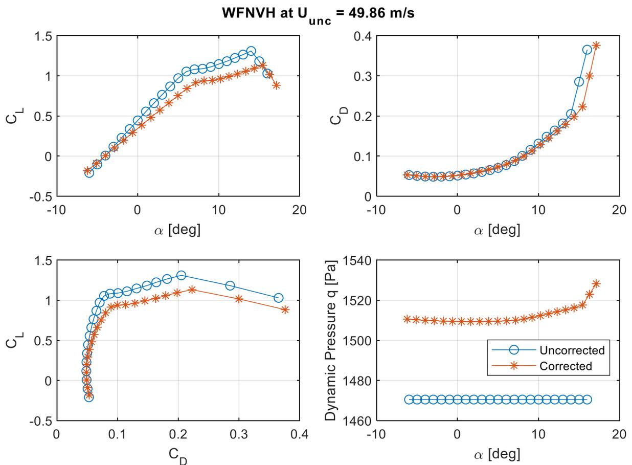
Figure 71: *WFNVH* Aerodynamic Parameters Values at  $U_\infty = 50 \text{ m/s}$ ,  $Re = 0.41 \cdot 10^6$ ,  $M = 0.145$
