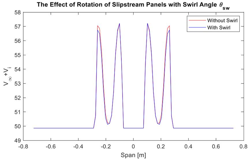
Figure 67: Effect of Swirl on the Axial Velocity Flowing Through the Propeller
