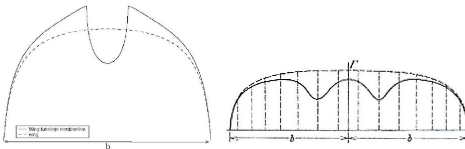
Figure 60: Fuselage Influence on Lift (Multhopp) (Left) [63] and Nacelle Influence on Lift (Durand) [39]
