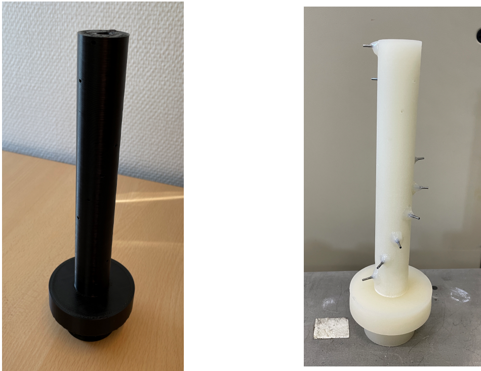
Figure 5.7: On the left, an example of one of the 5 3D printed PLA models, and on the right the 3D printed PP model where the metal tubes are glued in place. On the opposite side of the metal tubes are drilled holes, which are difficult to see.
