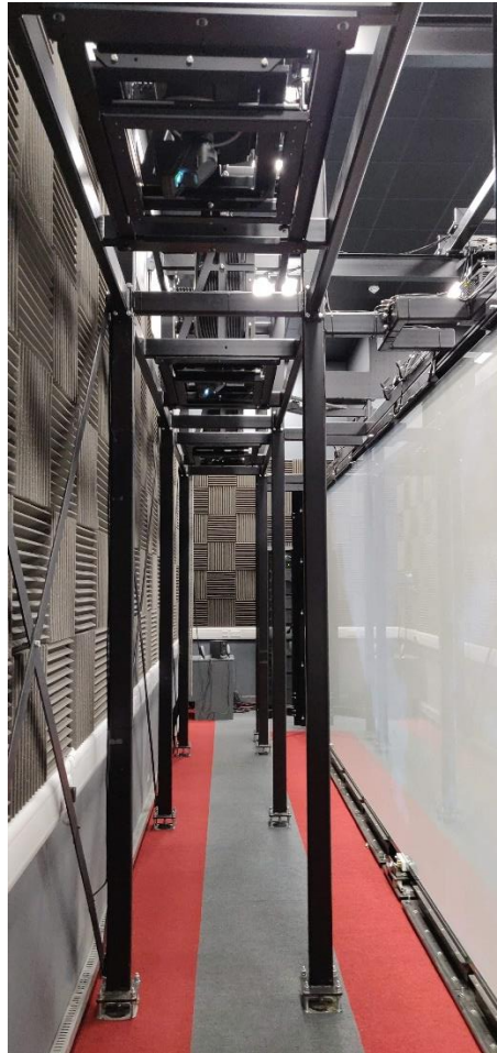
Figure 23. The left side of the HIKER where the projectors are fitted on a metal frame
