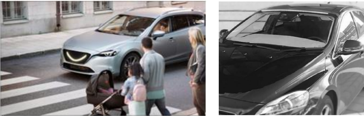
Figure 2: Left : Ego-centric information - Smile-shaped light bar on bumper showing pedestrians that it's OK to cross (image taken from Peters, 2016; Semcon, 2016). Right : Vehicle-centric information – AVIP (Autonomous vehicles' interaction with pedestrians) prototype which is a LED strip that lights up in different sequences to communicate that the vehicle is “in automated driving mode”, “is about to yield”, “is resting” or “is about to start” (copied from Habibovic et al., 2018; Lagstrom & Lundgren, 2015)
