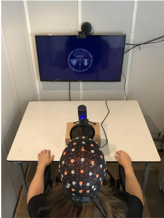
Fig. 1. Experimental set-up in the sound-attenuating room. The subject is wearing the EEG cap and sits in front of a microphone and a screen. The screen shows the visual cues during the experiment. In this illustrative figure, no visual cue is given.
