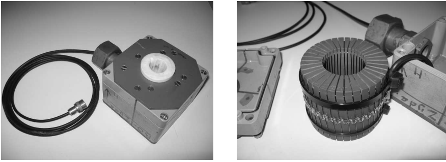
Figure 3.17: Left: the KEMA Rogowski coil as it is used in the measurements, right: the Rogowski coil outside its shielding box.
