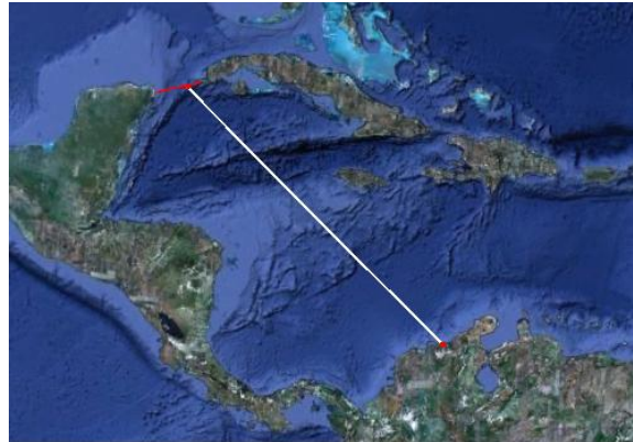
Figure 2.18: Maximum fetch of waves reaching the pass between Cuba and Mexico (Google Earth picture)
