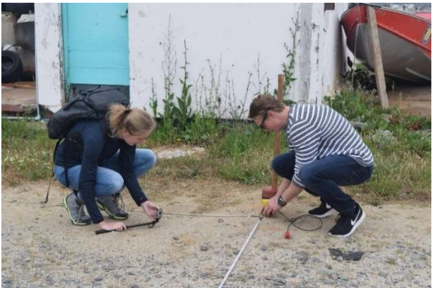
Figure C-12: Installing the geophones at 6m c.t.c. distance in L-shaped line
