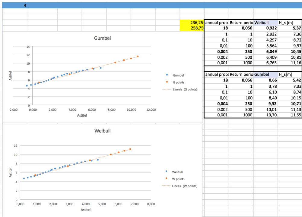
Figure H-2: SW swell waves, Gumbel and Weibull results and return period ave conditions
