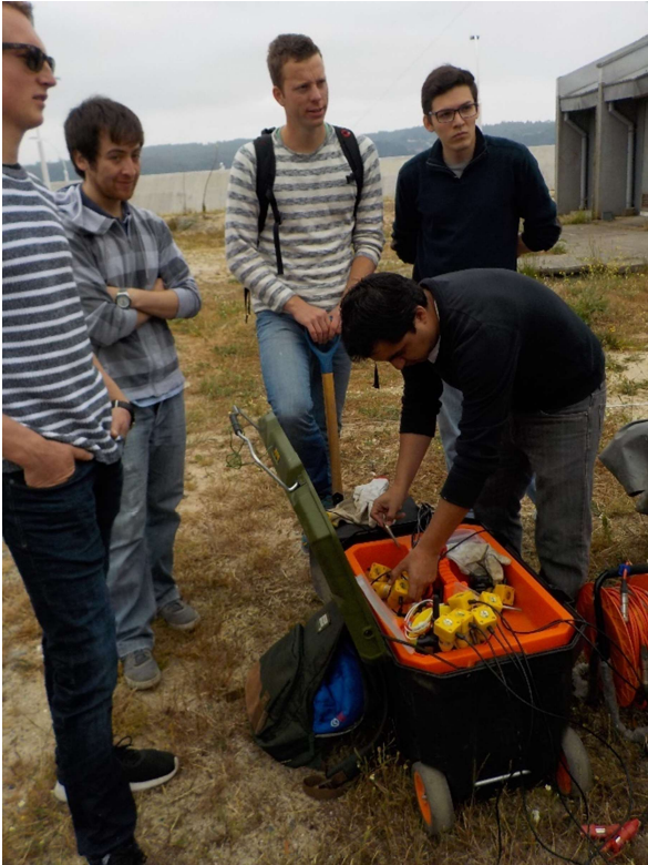
Figure C-11: Geophones (in yellow), installed in L-shape pattern on site
