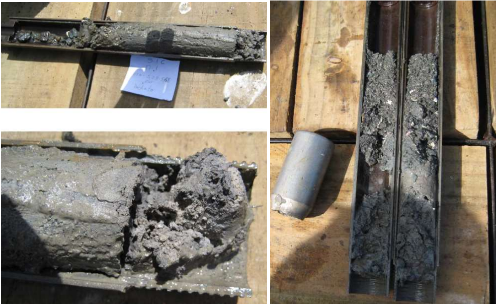
Figure B-3: Photographs of SPT samples from S-1 (left) and S-4 (right)
