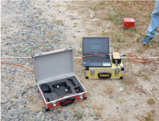
Figure C-13: Geophone recording set-up
