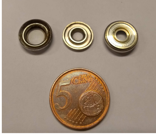
Figure 3.6.: Two Varioptic Arctic39N0 liquid lenses. The two parts on the left are the bottom and the top part of a lens showing the inside. The top half of the lens (middle) is coated entirely with a thin hydrophobic and insulating coating. The bottom half of the lens (left) contains a plastic ring that both seals the lens when pressed together with the bottom part and separates the top from the bottom electrodes similar to a button cell. A complete liquid lens is shown on the right.
