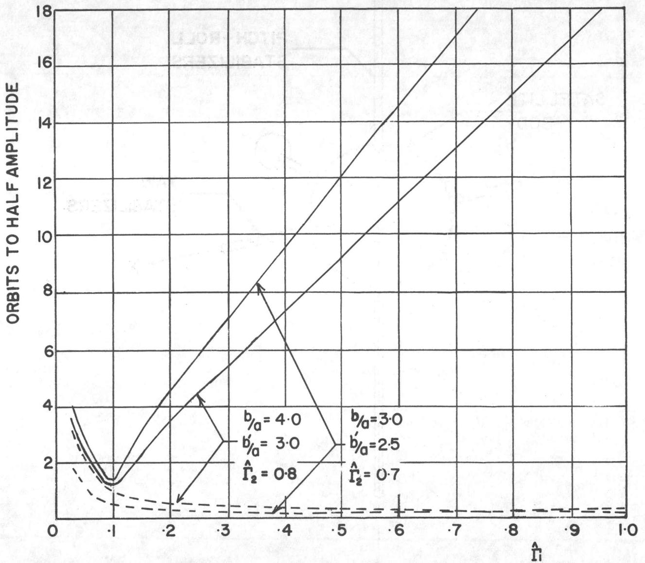
FIG. 5 DAMPING OF LEAST DAMPED MODE (GENERAL CASE)
