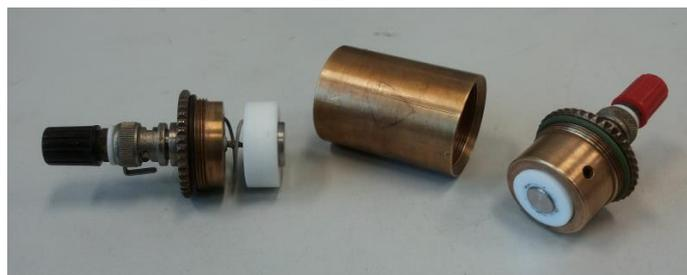
Fig. 11 Blocking cell used for impedance measurements of sample series HP and TF.
