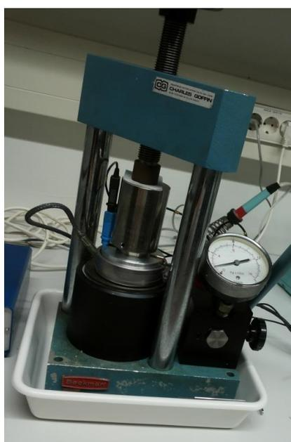
Fig. 12 Hand press combined with heating device used for impedance measurements in the press-cells (PC series). The press-cell is inserted in the heating block and connected to the Autolab.
