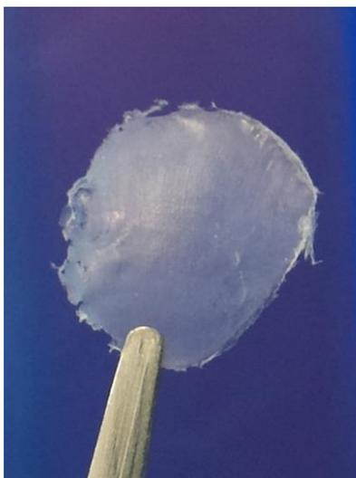
Fig. 18 One of the samples obtained by hot pressing in the cylindrical die set
