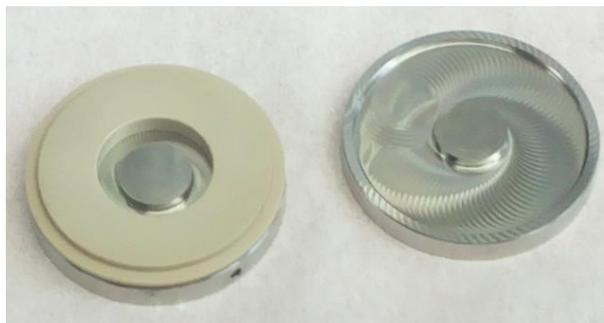
Figure 9 Picture of the open press-cell. The metal electrodes are in stainless steel, the white separator is in Peek.
