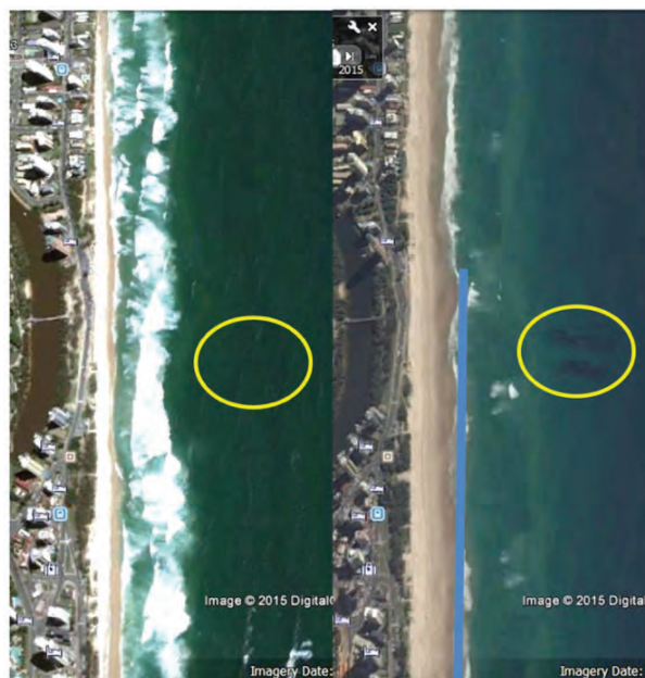
Figure 11. The Gold Coast Reef (Australia) constructed from 400 geotubes each 20m long
