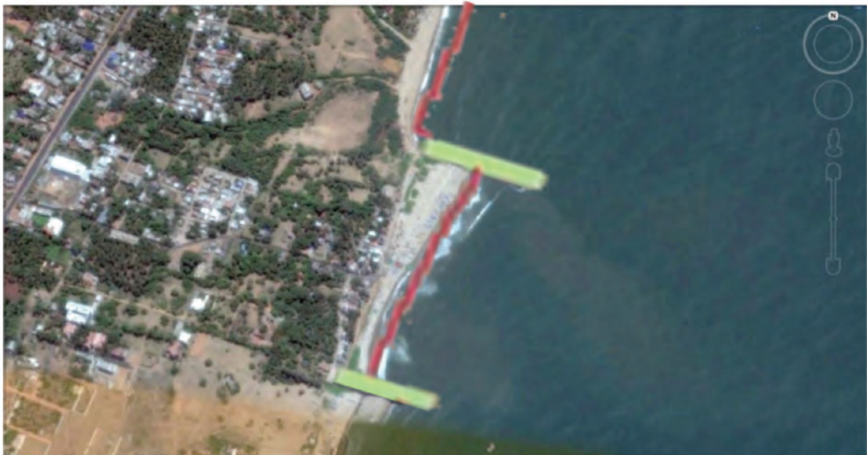
Figure 6. The Google Earth image overlaid with the shoreline position predicted by the computer model for July 3, 2014
