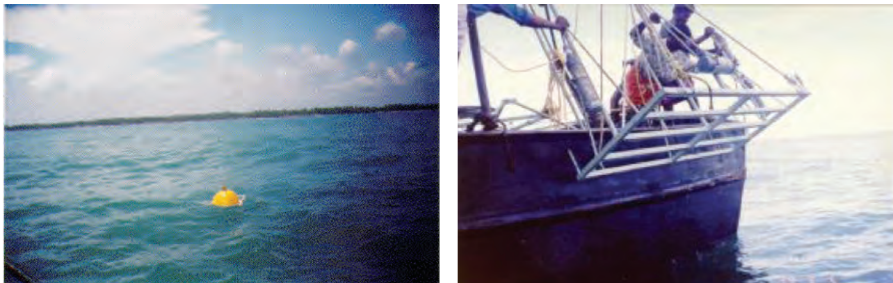
Figure 37. (Left) Directional wave-rider buoy deployed at the offshore site; (Right) sediment trap assembly being deployed at the site
