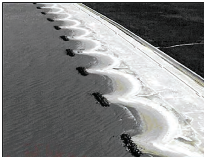
Figure 17. A series of offshore breakwaters with nourishment. The beach has formed into a pattern of salient and tombolos
