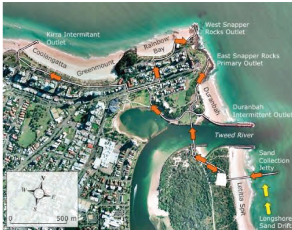
Figure 24. The Tweed River Entrance Sand Bypassing Project (TRESBP), Australia
