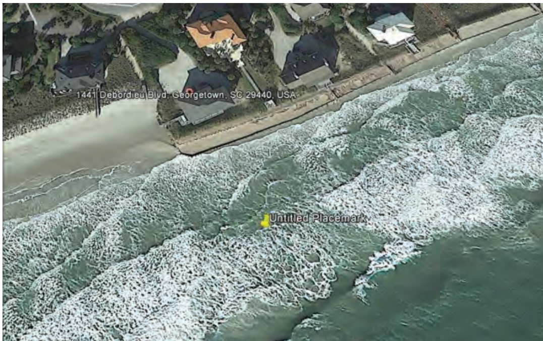
Figure 3. Typical seawall showing the end effect and loss of beach in front of seawall
