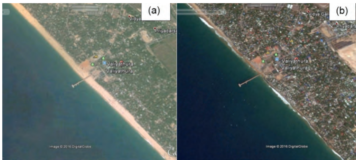
Figure 12. Valiathura coast: (a) 8/1/2003 and (b) 25/2/2016. Beach on either side of the pier including the northern side of seawall had 60-70m width in 2003. The seawall on the southern side was built after 2006, and by 2016 the beach vanished from the southern side
