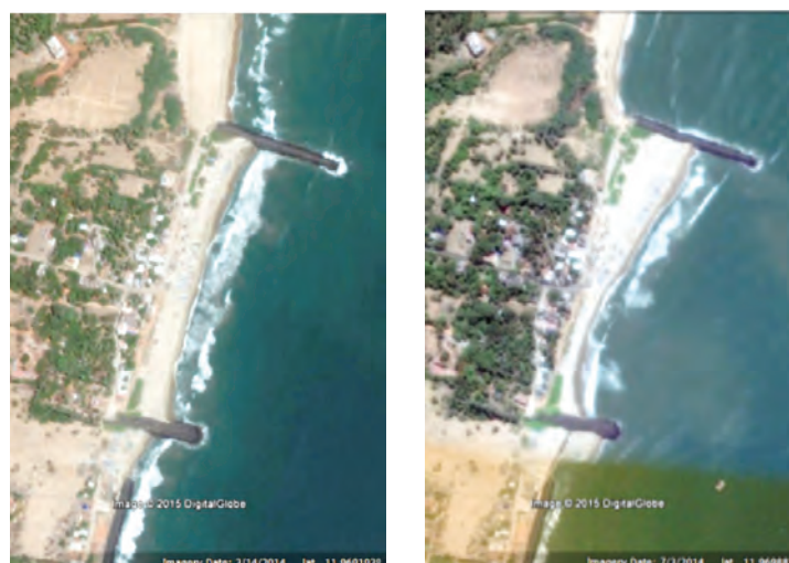
Figure 1. The beach in groyne compartments rotates seasonally in synchrony with the wave direction. The two yellow lines show the beach orientation after the NE monsoon and after the SW monsoon.
