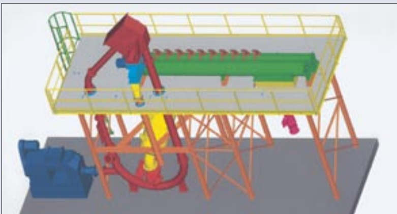
CAD drawing of the Delta Dryer test rig, a thermal dryer 8 metres high and 12 metres long, based on an idea of researcher Dr. Peter Rem.
