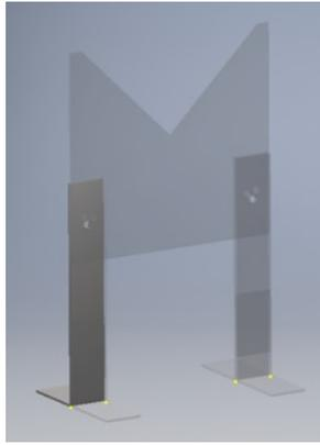
(a) V-Shaped design to elevate the pipe
