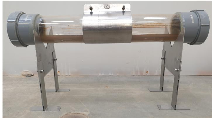
(b) The small-scale pipe on top of the two structures for elevation
