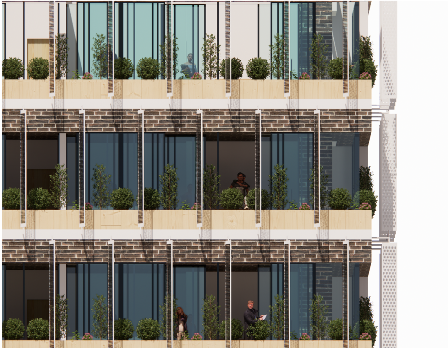
South facade with integrated BIPV panels in brise soleils
