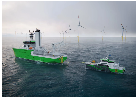
(b) Damen electric CTV getting charged from electric SOV
