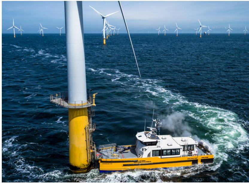
Figure 2.4: Catamaran CTV during maintenance execution [23]
