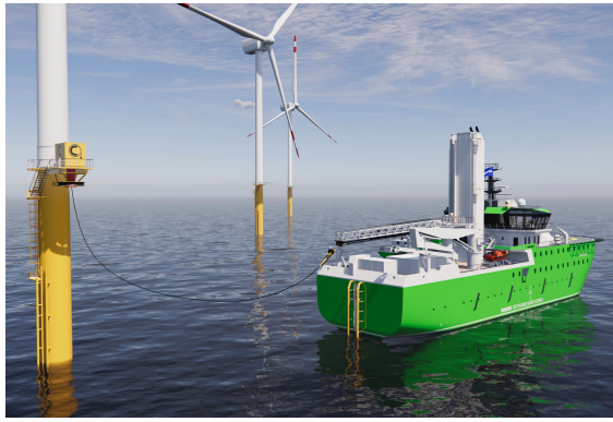
(a) Damen electric SOV charging concept
