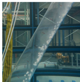
B - Two-layer flow, particles in suspension.
