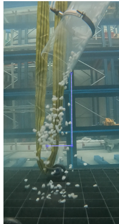
Figure 9.10: Measuring the offset at 25 cm below the pipe.
