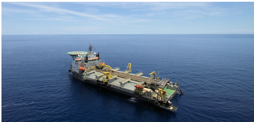
Figure 2.2: Side stone-dumping vessel NDeavor.
