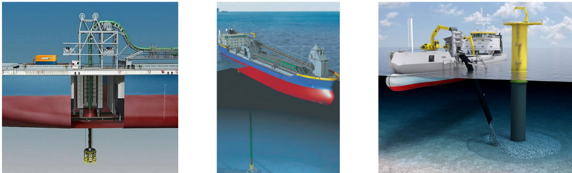
Figure 1.1: Three different methods of fall-pipe use: a flexible bucket system, a vertical fall-pipe and an inclined fall-pipe.
