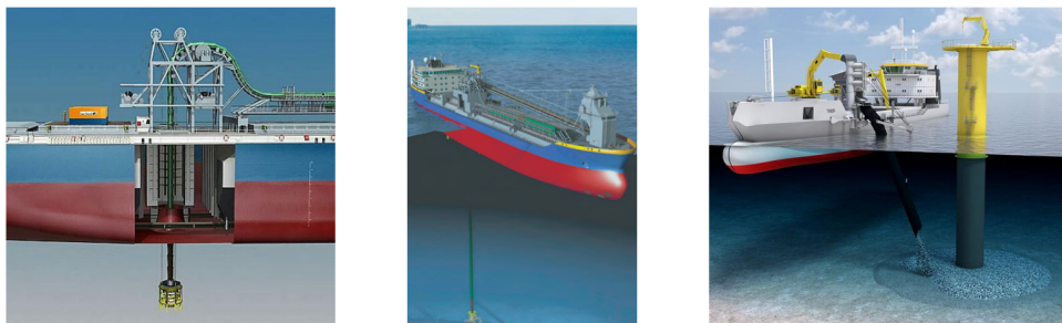
Figure 2.4: Three types of fall-pipe design: a flexible fall-pipe system, a closed fall-pipe and an inclined fall-pipe.
