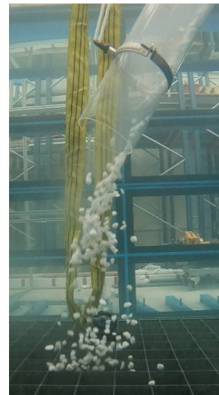
Figure 9.1: The cone shape of the rock mass (test 18).
