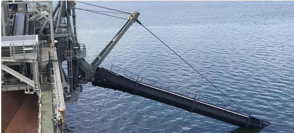
Figure 2.6: The inclined fall-pipe installed on the Rockpiper.
