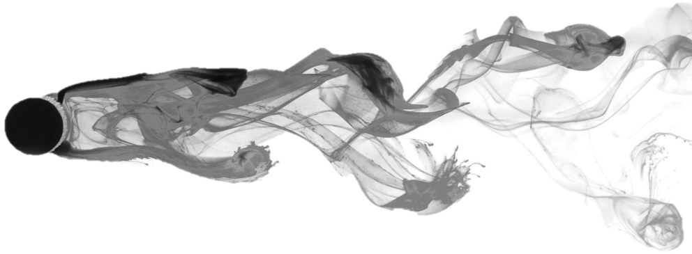
Figure 4.1: A Kármán vortex street behind a cylinder in water (Joseph Straccia, 2016).
