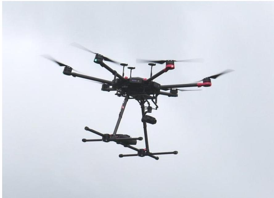
Fig.1: Photo of the M600, with its 6 propelled arms and 3 visible GPS antennas on top of the frame, equipped for a survey mission with the thermal camera and the geomagnetometer (attached to the landing skid).
