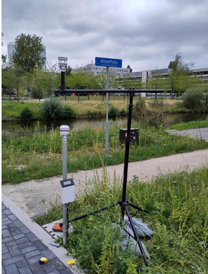
Figure 5: Two co-located anemometers are installed at station z6-20596 (August 25<sup>th</sup>, 2023)
