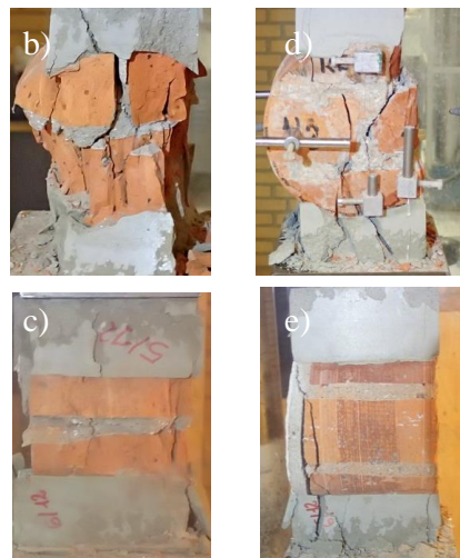
Fig. 13. Existing clay masonry (Rengersweg): (a) no information about crack pattern of wallets was available; (b)-(c) final crack pattern of T-shaped core; (d)-(e) final crack pattern of H-shaped core; (f) mean stress-strain relationships [45].
