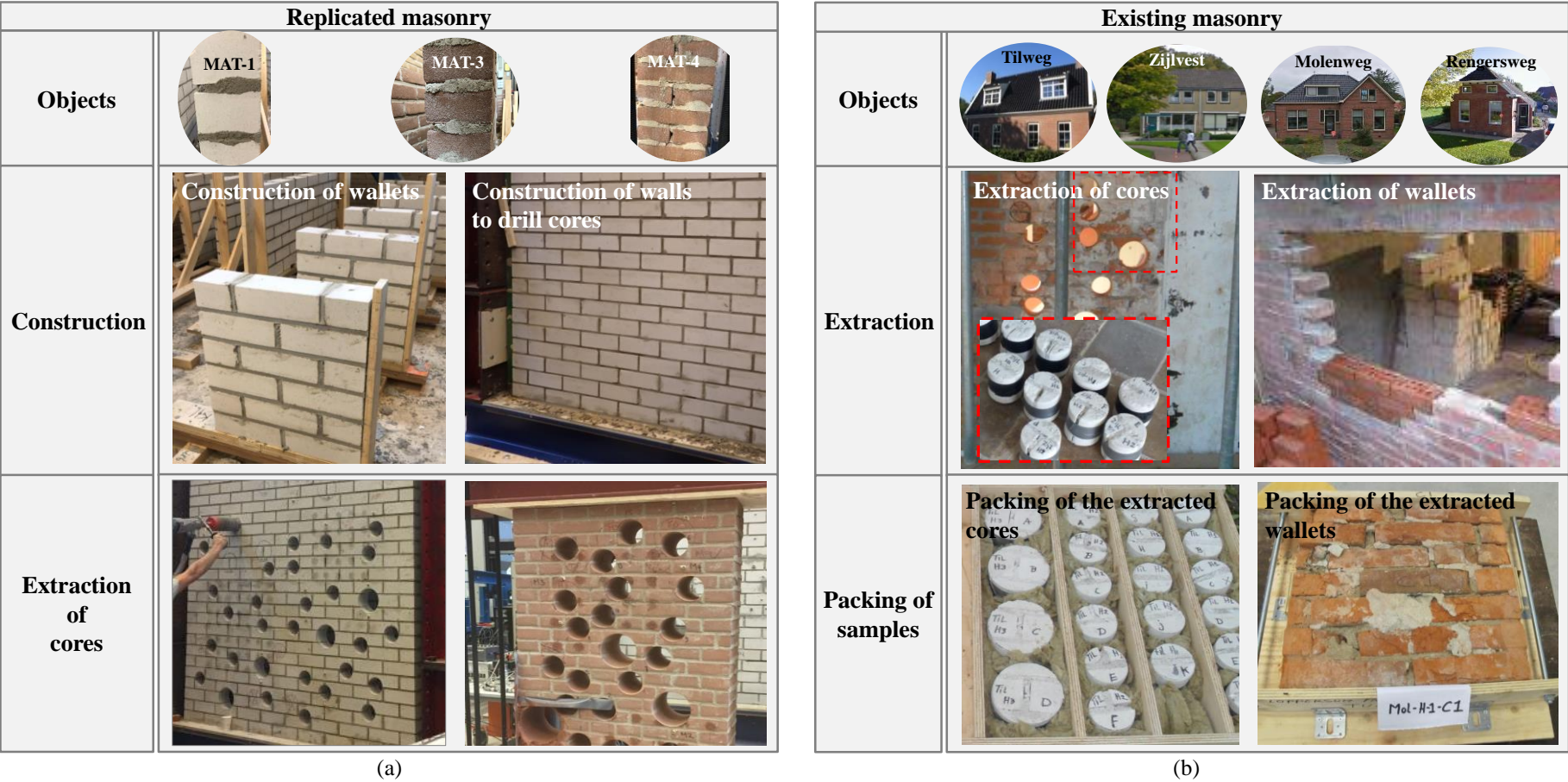
Fig. 1. Overview of the masonry objects: (a) replicated in laboratory; (b) extracted from existing buildings.
