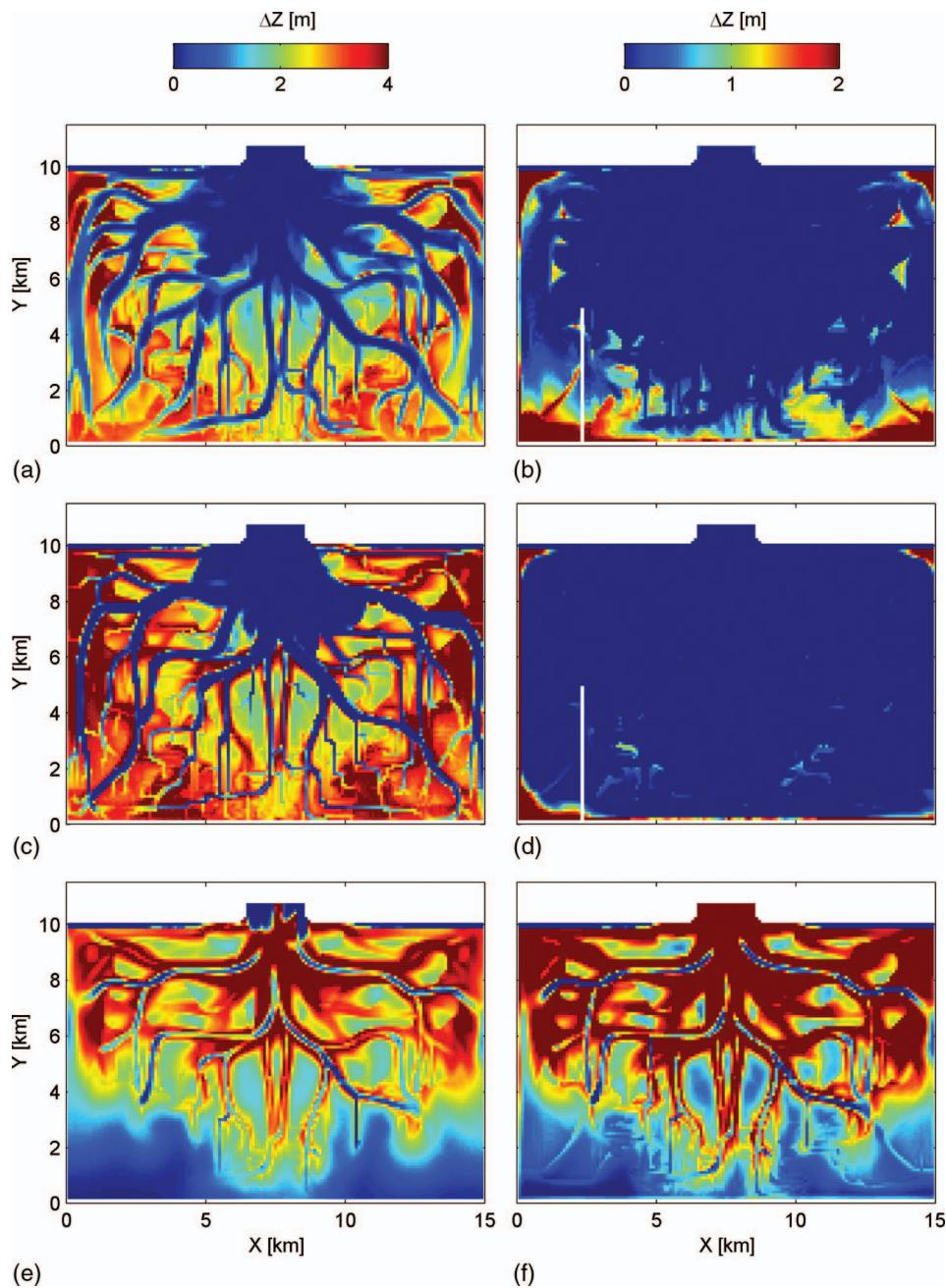
**Fig. 9.** (Color) Bed-level change after 25 years of mud infill; simulations (a, c, e) without waves; (b, d, f) with waves; (a and b) with the consolidation model; (c and d) with  $\rho_{\text{dry}} = 250 \text{ kg/m}^3$ ; and (e and f)  $\rho_{\text{dry}} = 800 \text{ kg/m}^3$ . Note the different scales in simulations with and without waves. The white lines in (b) and (d) depict the locations of model output shown in Fig. 10.
