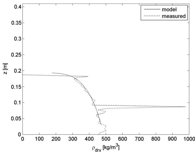
**Fig. 4.** Comparison of computed and measured density profiles at equilibrium for mud from Lake Markermeer.
