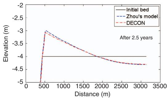
**Fig. 6.** (Color) Bed level after 2.5 years of simulation, computed with DECON and Zhou's model.
