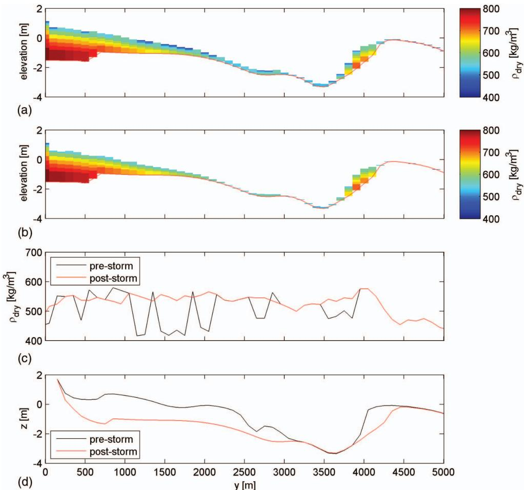
**Fig. 10.** (Color) Cross section of computed dry density: (a) before and (b) after a storm occurring in the 25th year of the model simulation; (c) the dry density of the near-surface layer for this simulation; and (d) the bed evolution of the model with low density and waves [corresponding to Fig. 9(d)] with the same pre- and post-storm conditions as (c). See Figs. 9(b and d) for the location of the transect.
