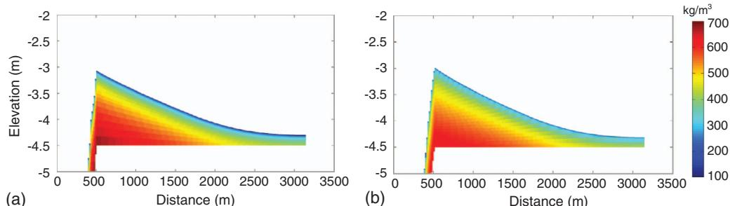
**Fig. 7.** (Color) Dry density distribution in the bed after 2.5 years of simulation: (a) DECON; and (b) Zhou's model.
