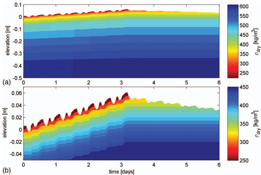
**Fig. 5.** (Color) Computed bed development at  $x = 2.5$  km with the complete bed profile and details near-surface with active and bed layers. The fluffy layer is not depicted (note different density scales).
