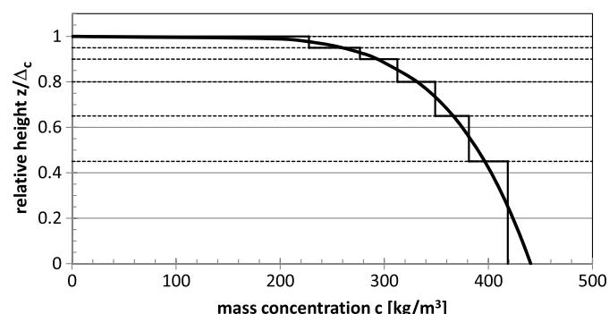
**Fig. 2.** Example of typical distribution of mass concentration at final consolidation with discretized distribution. The thick line represents an equilibrium density distribution, whereas the thinner staircased line represents the model's discretization.
