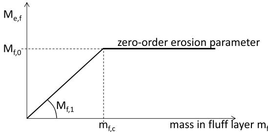
**Fig. 11.** Zero- and first-order erosion rates.
