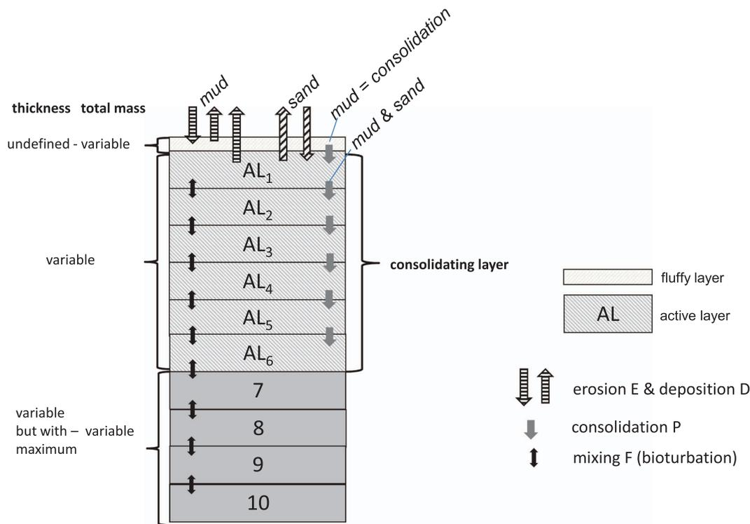
Fig. 1. (Color) Discretization of bed layers in the DECON model, modified from the generic bed model.
