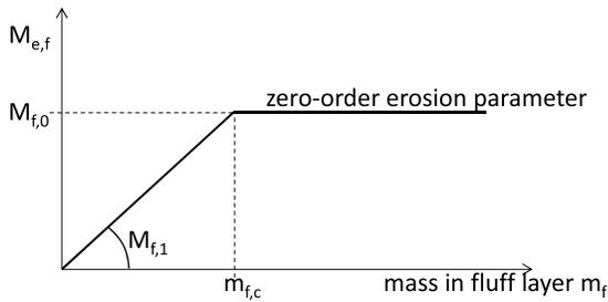
Fig. 11. Zero- and first-order erosion rates.
