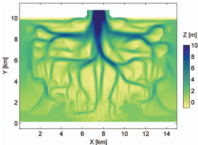
**Fig. 8.** (Color) Initial bed topography for the consolidation model, obtained from a 100-year morphodynamic simulation with 0.1 mm sand only and a 3 m symmetric tide at the inlet's mouth.
