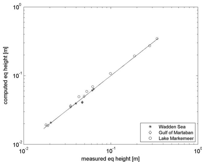
**Fig. 3.** Comparison of computed and measured equilibrium heights.
