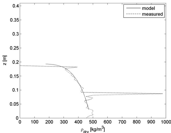
**Fig. 4.** Comparison of computed and measured density profiles at equilibrium for mud from Lake Markemeer.
