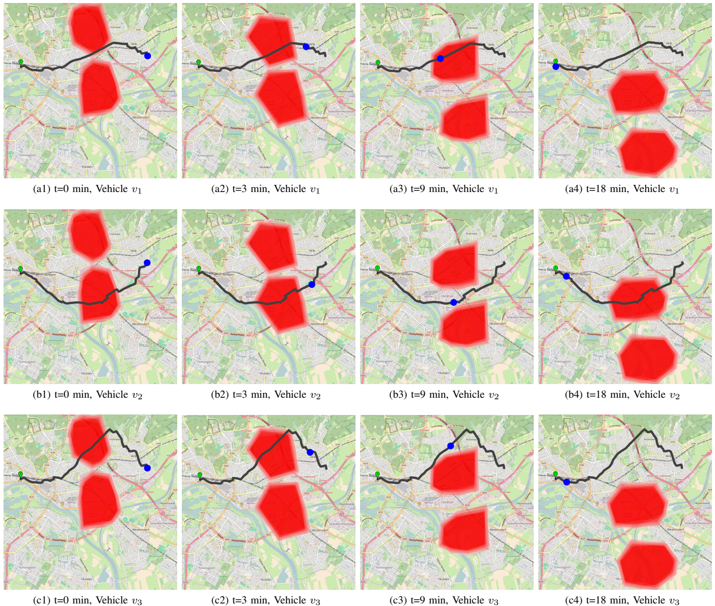
Fig. 15: Snapshots of routes calculated for 3 vehicles (in blue circle) with different categorization of risk levels. The vehicles are at the source points. The shapes and positions of the obstacles (in polygons) are the same in the three simulations, and will change as the vehicles are moving towards the destinations. (a) Vehicle v_1 , full-safe levels ={L0, L1, L2}, partial-safe levels ={L3, L4, L5}, non-safe levels = \emptyset . (b) Vehicle v_2 , full-safe levels ={L0, L1}, partial-safe levels ={L2, L3}, non-safe levels = {L4, L5}. (c) Vehicle v_3 , full-safe levels ={L0}, partial-safe levels ={L1}, non-safe levels = {L2, L3, L4, L5}.
