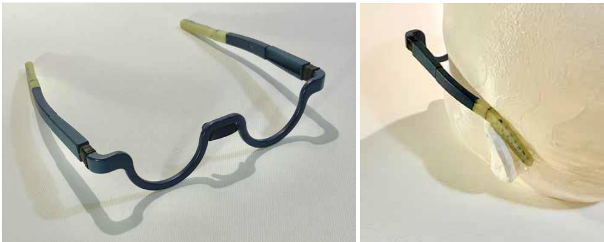
Figure 5: Special tool designed to measure the geometry behind the ears
