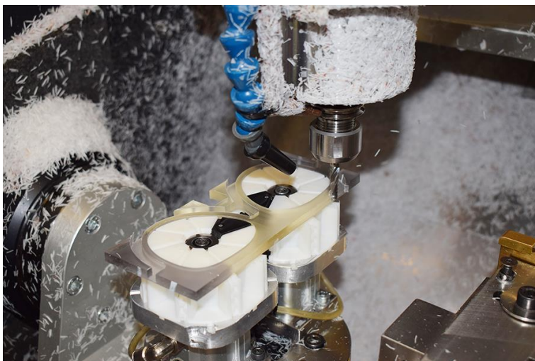
Figure 3: Milling process of acetate glasses
