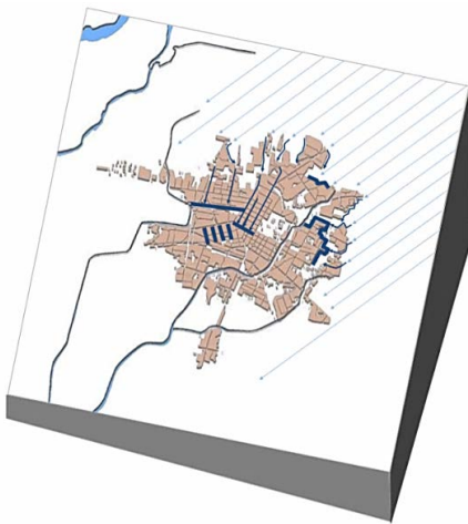
Flow way has changed when urban constructions block the ways
