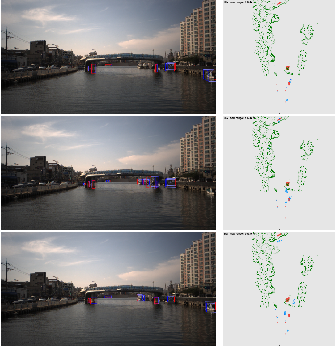
Figure A.2.16: Qualitative detection results on sample 1 for GaussianFusion under different uncertainty scale factors: \alpha = 0.1 (top row), \alpha = 0.05 (middle row), and \alpha = 0.2 (bottom row). Each row shows the camera view (left) and the corresponding BEV (right). Refer to Figure A.2.1 for the ground truth annotations.
