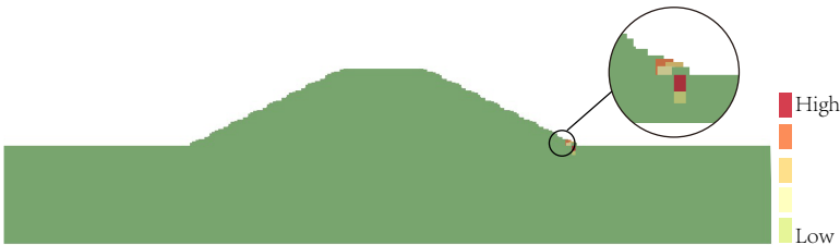
Figure 6.10: Locations of the points with maximum local velocity from 500 realisations ( COV_k = 0.1 and \xi = 1 ).
