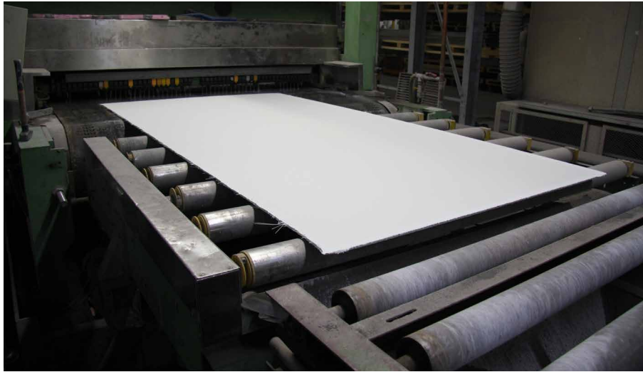
FIGURE 6.1 Automated production process for flat thin-walled GFRC (shown panel size ca 4m x 1.2m).
