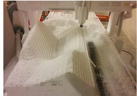
FIGURE 4.8 Concrete mould milled by a CNC machine
