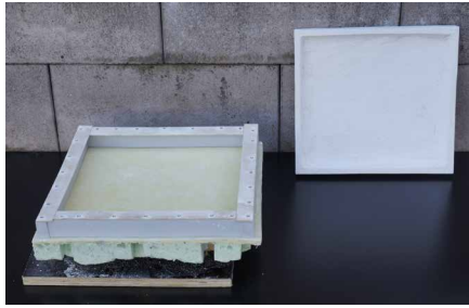
FIGURE 7.4 Intermediate mould with high edge-return
