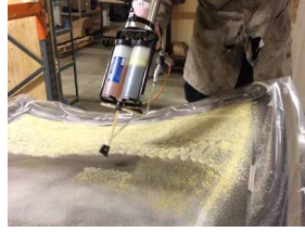
FIGURE 5.15 Casting the foam mould on the shape
