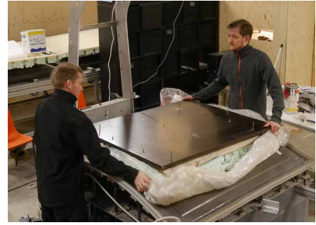
FIGURE 6.22 Final demoulding of the intermediate mould, before the edges are being trimmed and the edge-barrier being fitted.
