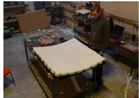
FIGURE 6.24 Finished intermediate mould ready for being tested with sprayed GFRC.
