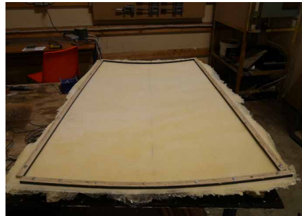
FIGURE 6.13 Fitting timber edges barriers on the mould
