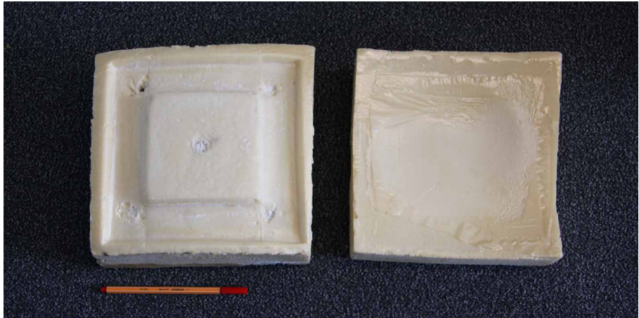
FIGURE 6.8 Small scale (23cm x 23cm) sample two-part intermediate mould for use with the premixed method.
