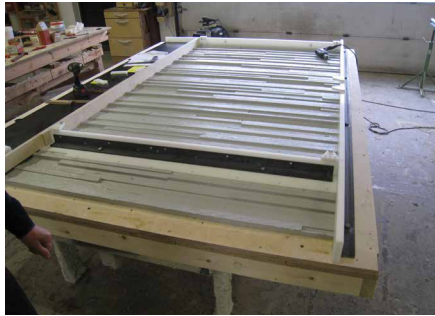
FIGURE 4.3 Flat rubber mould with a texture finish
