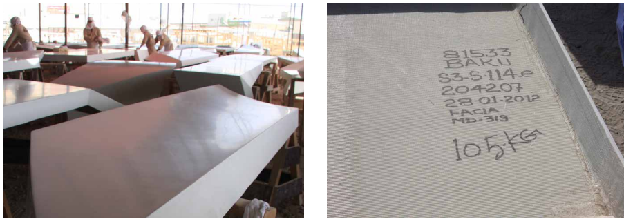
FIGURE 3.4 Production of GFRP cladding panels for the Heydar Aliyev Center
