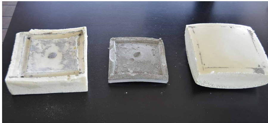
FIGURE 4.14 The first cast proto type utilizing the new mould system
