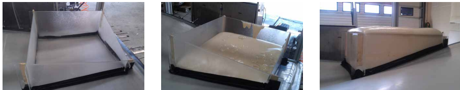
FIGURE 3.10 The proposed new approach which adds an additional step between the flexible table and the casting of the GFRC element.
