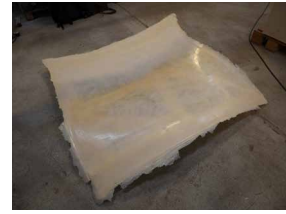
FIGURE 5.16 Completed mould & finished surface
