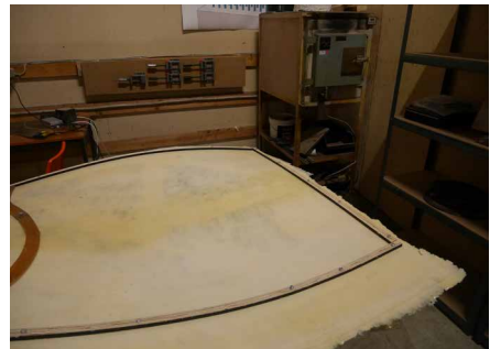
FIGURE 6.17 Fitting edges on the mould
