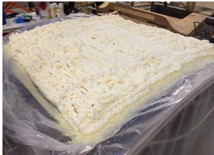
FIGURE 6.12 Curing the LDPU on the flexible table
