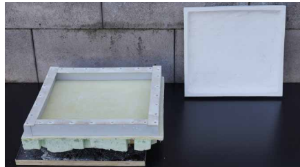
FIGURE 6.25 Intermediate mould with high edge-return
