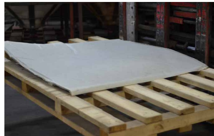
FIGURE 6.3 The automated premixed GFRC panel after curing and removal of protective foil. Panel is 1,2m x 1,2m.
