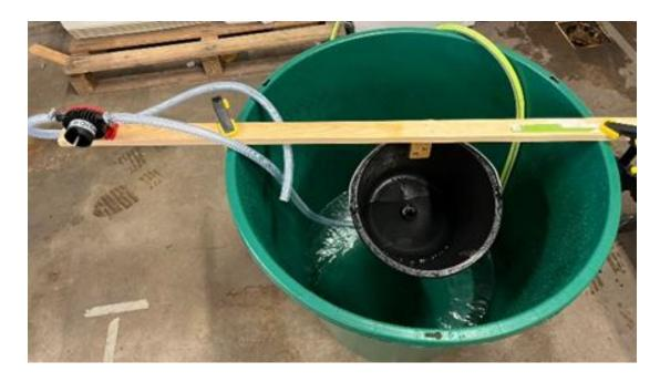
Test set up with 1300 l/h pump
