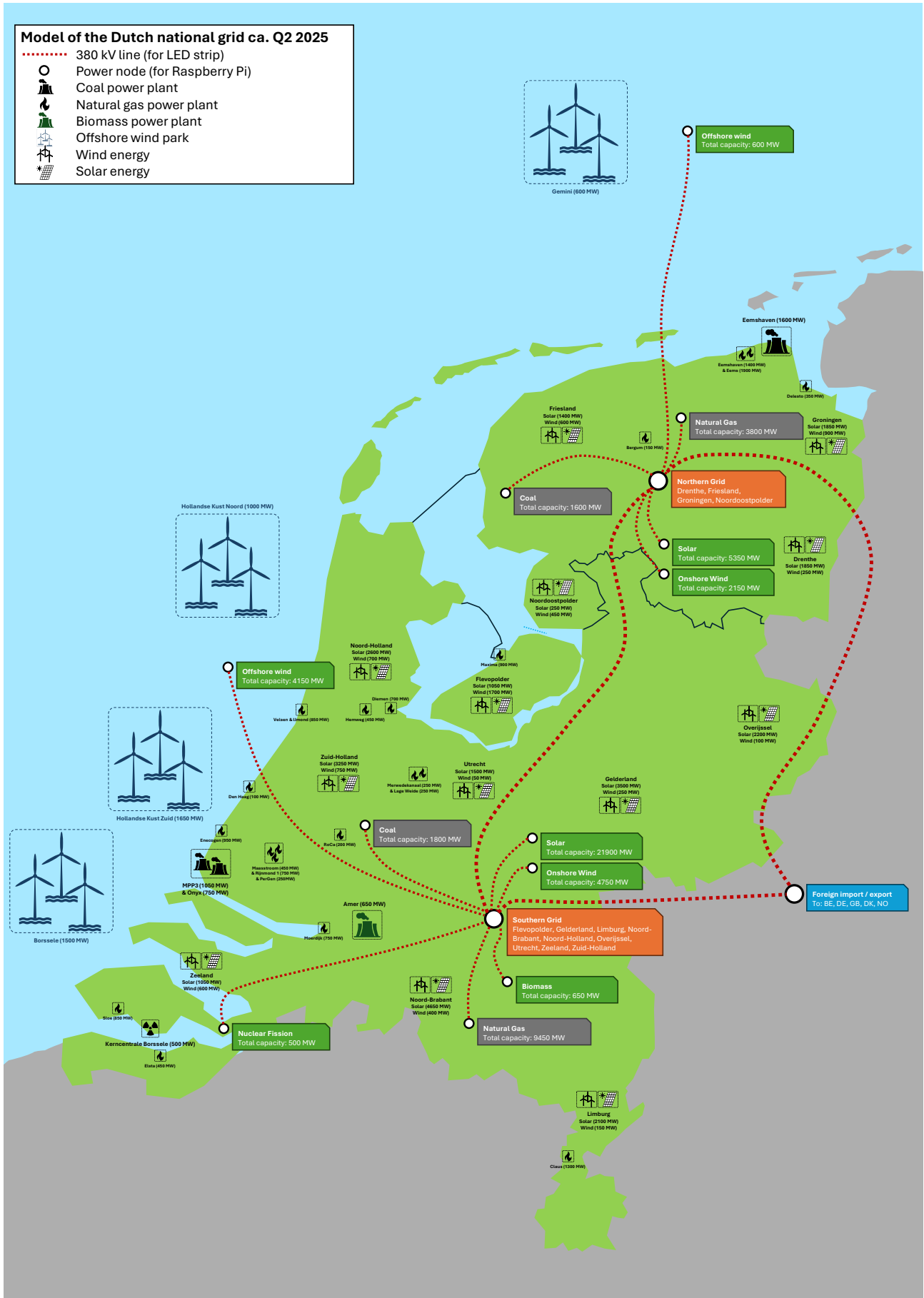
Figure 3.14: A stylized version of the simplified grid model. This figure is intended to be printed on 9 A3 papers. Raspberry Pi's with the Illuminator software can be placed on the circles to run the model.
