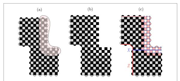
**Figure 11.** (a) The layout where the qubits in the region highlighted are each to be measured in the X basis. (b) The stabilizers of the underlying subsystem code C. (c) The gauge operators (in red) and logical operators of the code. One can see that the distance is guaranteed by the amount of overlap between the two blocks. The distance of the subsystem code is 4.
