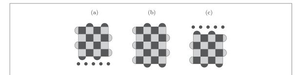
**Figure 2.** A procedure to flip a lattice using code deformation. (a) The lattice to be flipped, and the physical qubits prepared in  $|+\rangle$  states. (b) The flip operation is realized by merging the original lattice with the physical qubits below. (c) Subsequently measuring the physical qubits at the top in the *X* basis finishes the flip operation.
