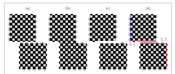
**Figure 10.** (a) and (b) The qubit layouts before and after the plain merge operation. The number of logical qubits is kept constant during this merge operation. (c) The stabilizers of the subsystem code. (d) The gauge operators and logical operators of the subsystem code. One can see that the distance is guaranteed by the offset between the two blocks. The distance of the separate surface codes is 11, and the distance of the subsystem code is 4.
