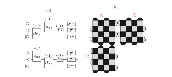
**Figure 4.** (a) Two equivalent measurement-based circuits for the CNOT gate. (b) The qubit layout for a CNOT gate between two surface-code qubits. C is the control qubit, T is the target qubit, and A is a logical ancilla.
