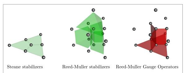
**Figure B1.** Stabilizers of the Steane and Reed–Muller codes, and Z gauge operators of the Reed–Muller code. Red tinting on a face or volume indicates the presence of a Z operator on the vertices which make up that face or volume. For example, there are six Reed–Muller gauge operators of the form  $Z^{\otimes 4}$ , supported on the red-tinted quadrilaterals seen on the right. Green tinting indicates the presence of both an X and a Z stabilizer operator.
