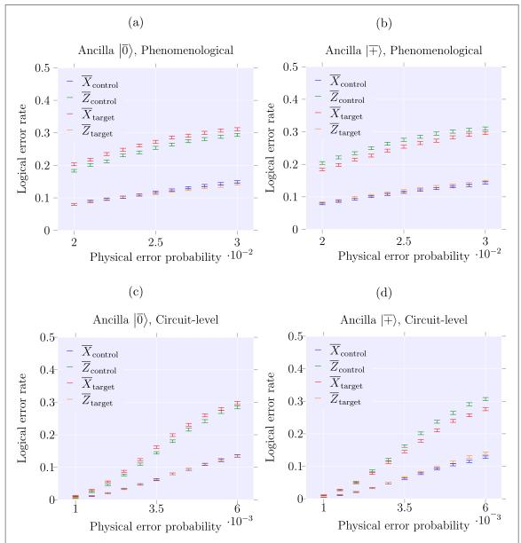
Figure C2.  $\overline{X}$  and  $\overline{Z}$  error rates on the control and target qubits for lattice-surgery-based CNOT operations at distance 5. (a) and (b) Correspond to the phenomenological error model, (c) and (d) correspond to the circuit-based error model. The disparity in error rates is explained by error propagation through the measurement-based circuit implementing the CNOT.
