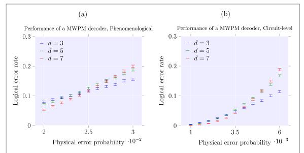
Figure 13. Numerical simulations of a fault-tolerant memory operation with the phenomenological error model near its threshold ( $\sim$ 2.75% (a)) and the circuit-level error model near its threshold ( $\sim$ 0.5% (b)).
