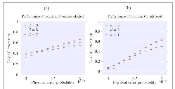
Figure 15. Numerical simulations of the rotation procedure in figure 1 without a final flip operation. (a) and (b) The logical error rates of the rotation procedure with phenomenological error model (the error threshold is around  $\sim$ 2.5%) and circuit error model (the error threshold is around  $\sim$ 0.45%), respectively.
