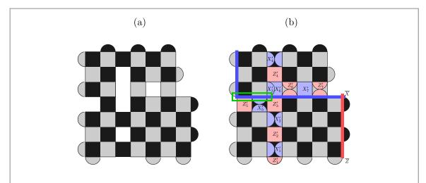
**Figure 8.** The operators of the subsystem code for the one-step grow operation from figures 1(a) to (c), skipping figure 1(b): (a) the stabilizers which generate S and (b) the whole gauge group, G, with highlighted gauge operators and logical operators.
