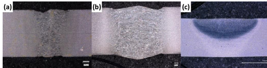
Fig. 3.31. Optical microscopic top view of the fusion zone welded by laser beams with a spot diameter of (a) 0.2 mm, (b) 0.6 mm, (c) 1.2 mm, a power of 4000 W, an incident angle of 90^\circ and a travel speed of 40 mm/s.
