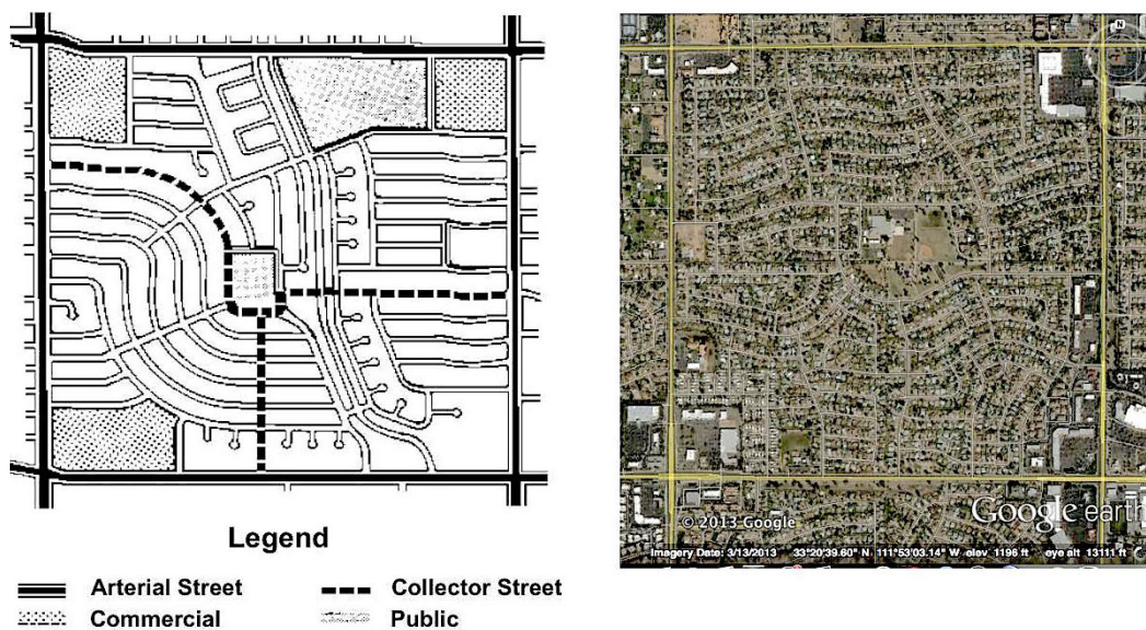
FIGURE 5.2 The Neighborhood Unit integrated with the US Functional Classification System (left) which became the model for development in cities like Phoenix (right). Areas of minimum ½ mile in width interrupted through traffic, which was concentrated in perimeter arterials. Central uses were limited to neighbourhood institutions, like parks and schools. The perimeter arterials fed largely discontinuous collectors, which led into highly discontinuous local streets. Sources: fhwa.gov, Google Earth.
