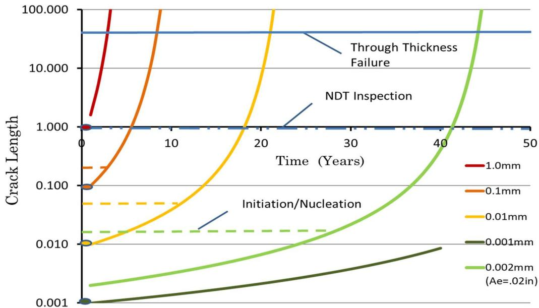
Figure 6.2 – Fatigue crack growth rate sensitivity to initial flaw size
