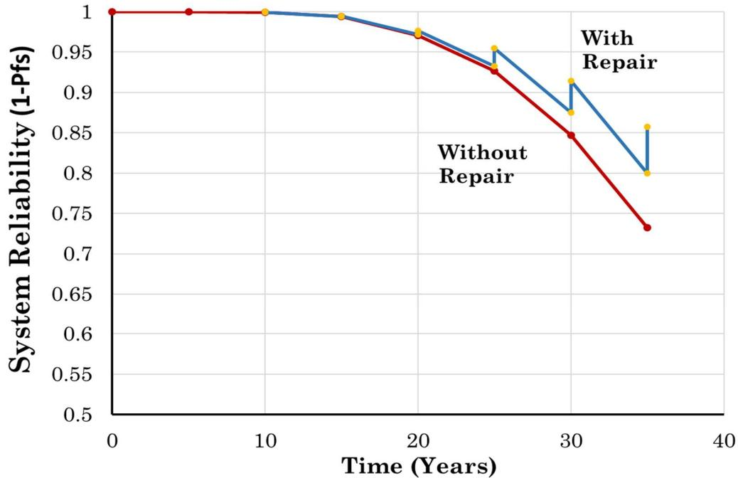
**Figure 2.6 – Example ship structure fatigue system reliability with updating**
