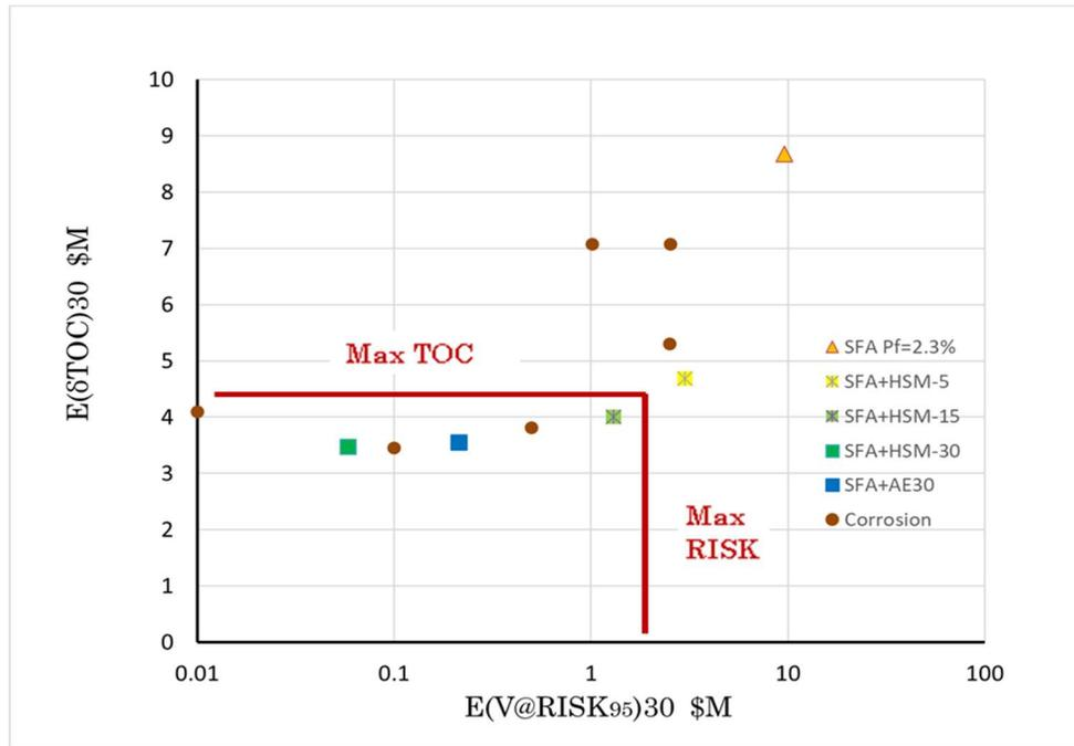
**Figure 6.19 – Illustration of RISK - TOC trade-off space for determining EOSL**
