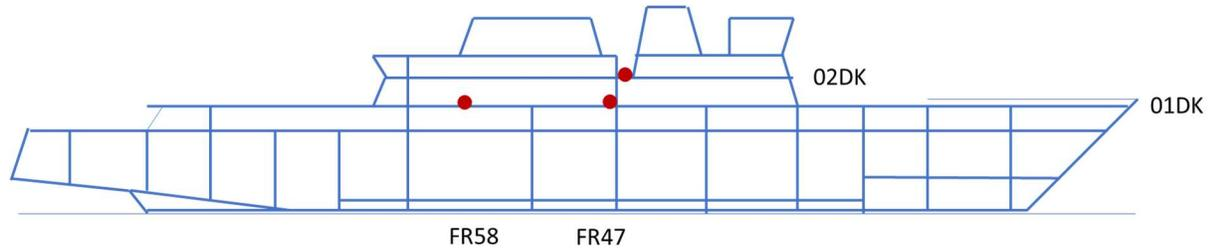
**Figure A.1 Illustration of the cutter's Inboard Profile with frame and deck locations.**
