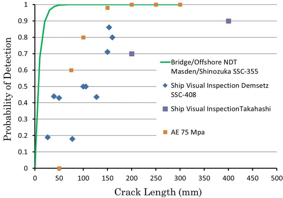
**Figure 6.13 – Probability of Detection for fixed structures and ships**
