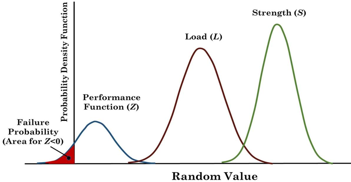
**Figure 2.3 – Illustration of fatigue reliability calculation (Redrawn from Ayyub *et al.*, 2014)**
