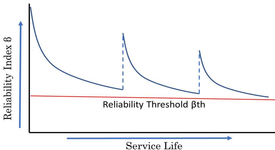
**Figure 3.1 – Illustration of Optimal Inspection and reliability updating**
