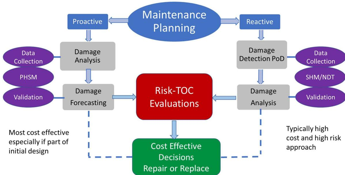
**Figure 5.13 - Comparison of reactive and proactive monitoring and maintenance approaches**
