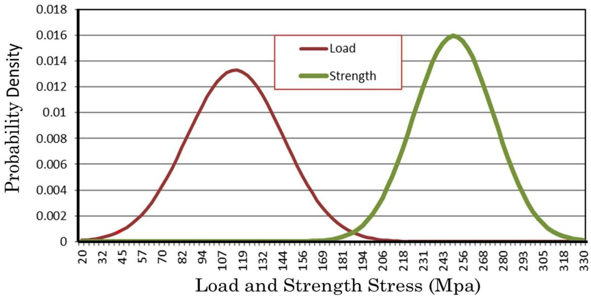
**Figure 6.3– Illustration of the Load-Strength interference calculation**
