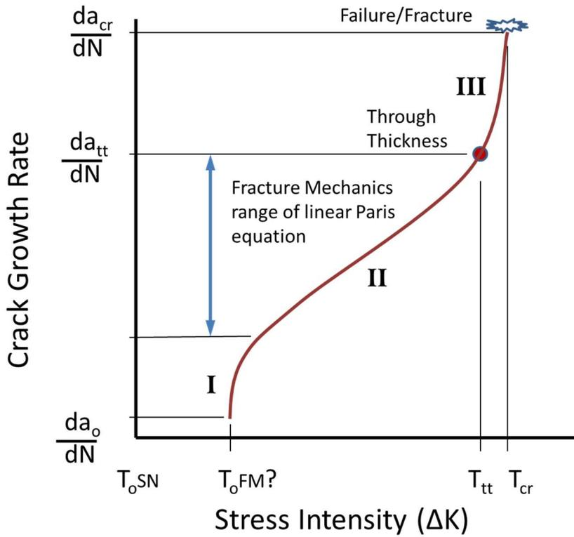
Figure C.2 – Illustration of the relationship between the F-M approaches for fatigue crack length over time.
