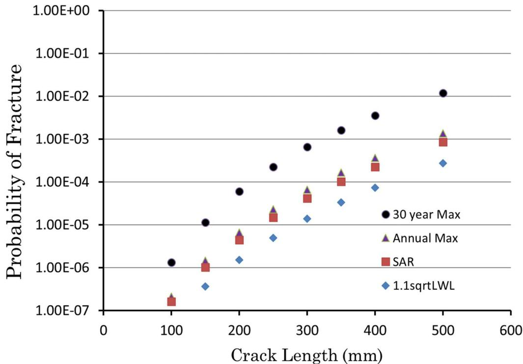
**Figure 6.4 – Estimated probability of failure for various loading conditions and crack lengths**
