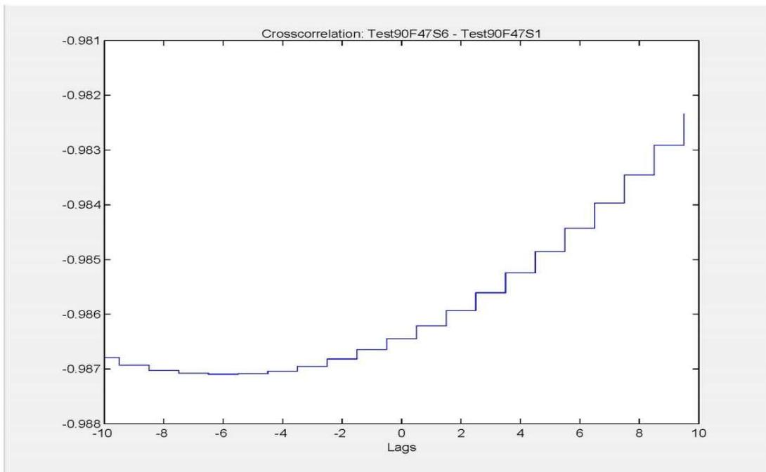
**Figure A.7 – Test 90 Cross-Correlation plot of F47S1 and F47S6 strain measurements**
