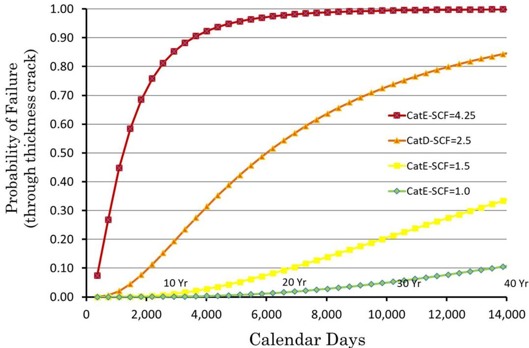
**Figure 2.4 – Example fatigue failure ( $ttc$ ) estimate for critical details in a ship hull structure with correlated groupings according to stress concentration factors and fatigue categories**
