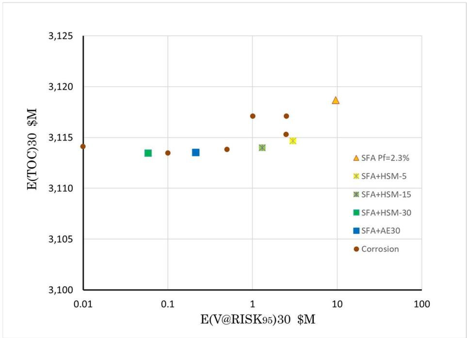
Figure 6.17 – Risk-TOC trade-space with fatigue and corrosion risk control scenario's
