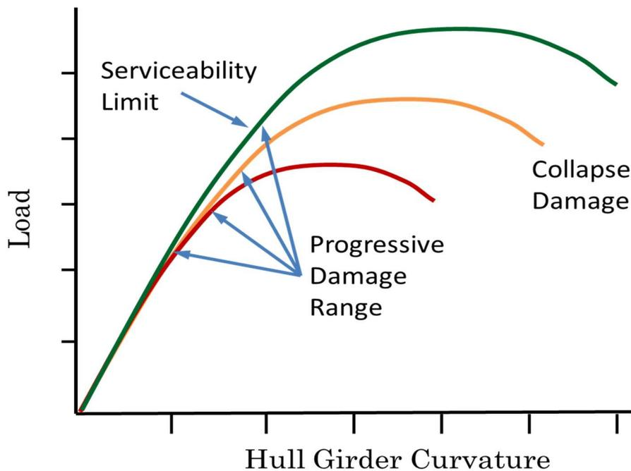
**Figure 2.1 – Illustration of load and hull curvature showing transitions from serviceability limit state to ultimate failure limit state**
