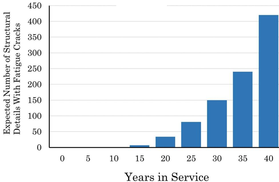
**Figure 2.5 - Expected number of ship hull structural details with *ttc* fatigue cracks**
