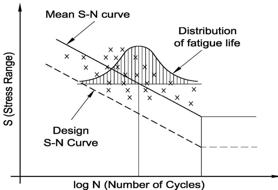
**Figure 2.2 - Illustration of characteristic design curve and test data (redrawn from Hughes *et. al.*, 2010)**
