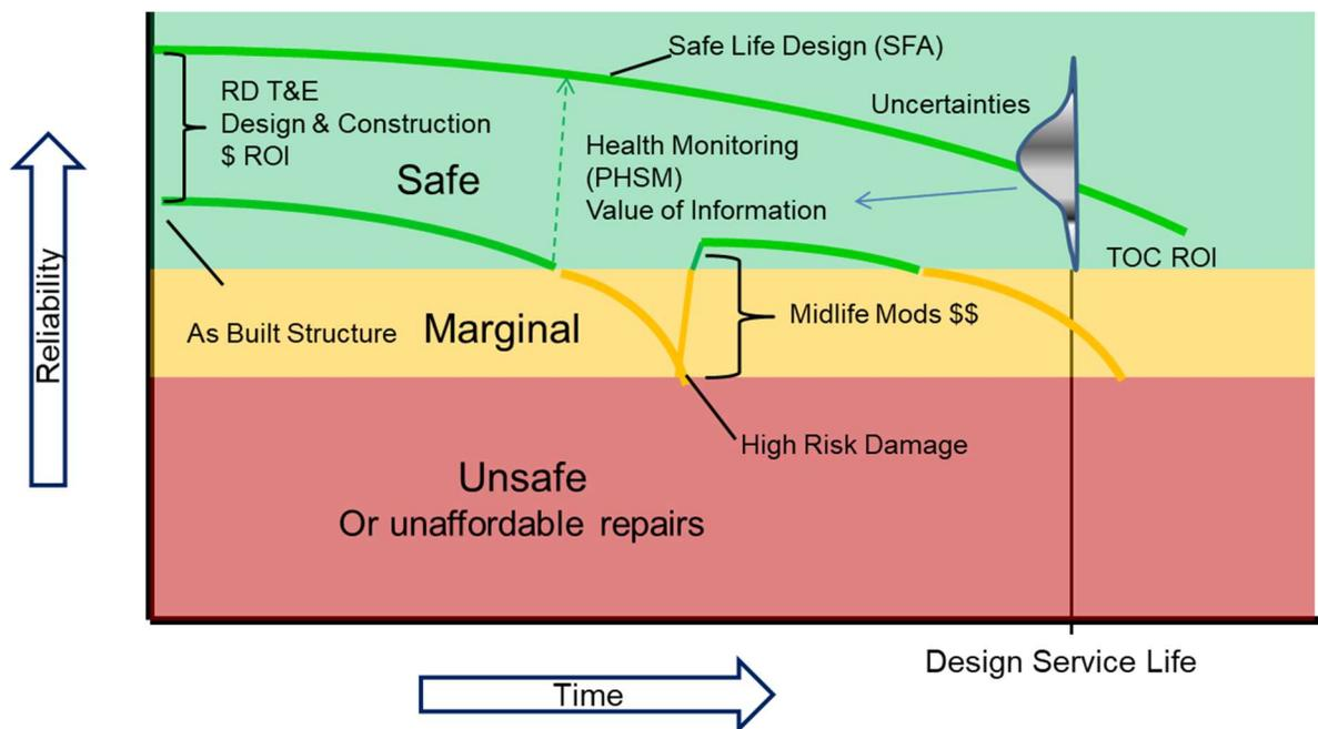
**Figure 6.5 - Illustration of structural reliability as a function of time with SFA and HSM**
