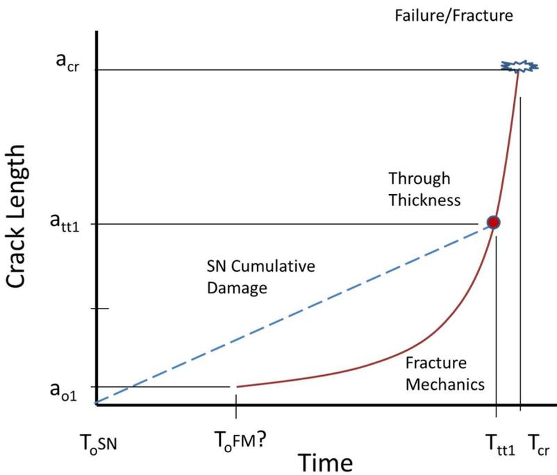
Figure C.3 - Relationship between the S-N+F-M Total Life approaches for fatigue crack length as a function of time.
