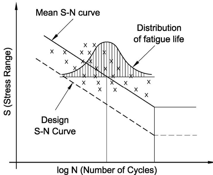
**Figure C.1 - S-N data used for fatigue crack initiation to through-thickness crack based on stress cycles to failure (Redrawn from Hughes 2010).**
