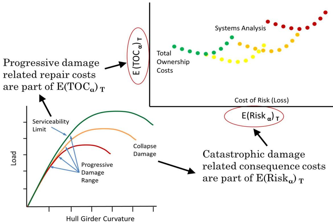
**Figure 5.11 - Relationship of serviceability failure and ultimate failures as part of TOC and Risk respectively**
