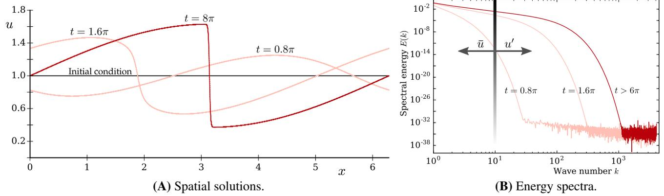
**FIGURE 3** Direct numerical simulation solution of the Burgers problem at different time instants. A, Spatial solutions; B, Energy spectra [Colour figure can be viewed at [wileyonlinelibrary.com](http://wileyonlinelibrary.com)]
