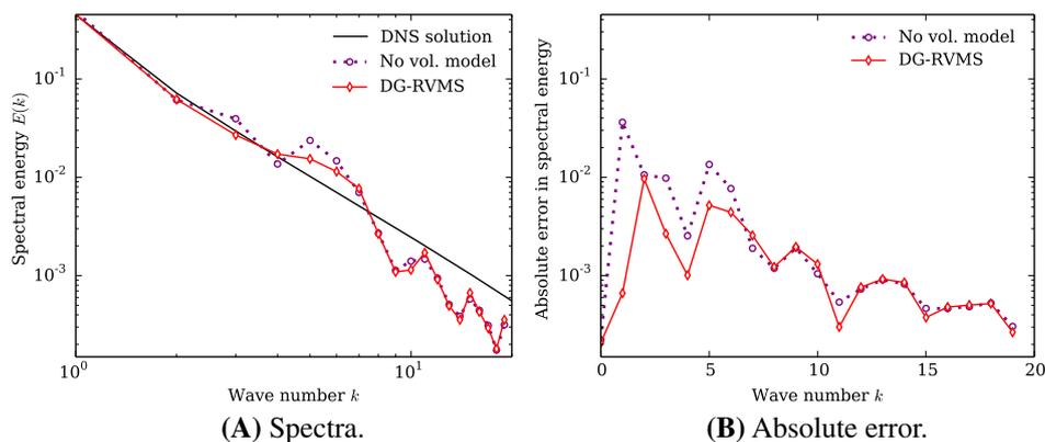
**FIGURE 13** Spectral energy obtained with four discontinuous Galerkin elements of  $p = 4$  and 20 degrees of freedom. A, Spectra; B, Absolute error. DG-RVMS, discontinuous Galerkin residual-based variational multiscale; DNS, direct numerical simulation [Colour figure can be viewed at [wileyonlinelibrary.com](http://wileyonlinelibrary.com)]
