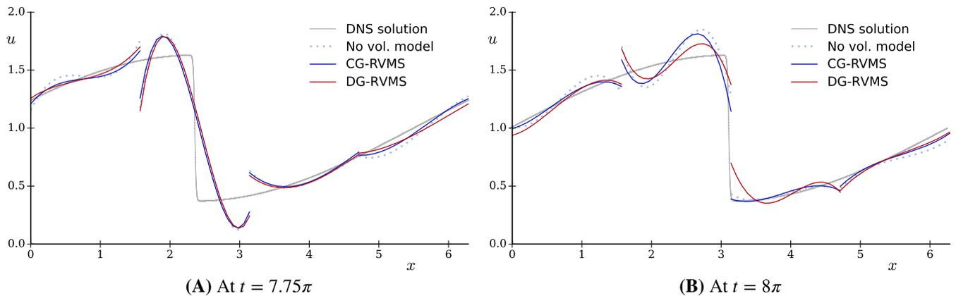
**FIGURE 6** Example solutions with and without the proposed discontinuous Galerkin residual-based variational multiscale (DG-RVMS) model, using four discontinuous Galerkin elements of  $p = 3$ . A, At  $t = 7.75\pi$ ; B, At  $t = 8\pi$ . CG-RVMS, continuous Galerkin residual-based variational multiscale; DNS, direct numerical simulation [Colour figure can be viewed at [wileyonlinelibrary.com](http://wileyonlinelibrary.com)]
