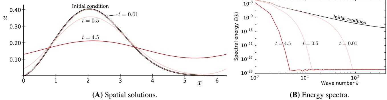
**FIGURE 1** Solution of the diffusion equation at different time instants. A, Spatial solutions; B, Energy spectra [Colour figure can be viewed at [wileyonlinelibrary.com](http://wileyonlinelibrary.com)]
