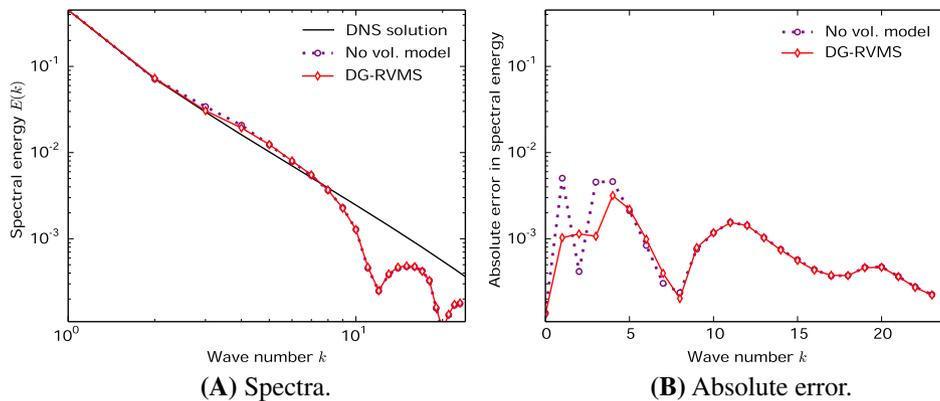
**FIGURE 11** Spectral energy obtained with eight discontinuous Galerkin elements of  $p = 2$  and 24 degrees of freedom. A, Spectra; B, Absolute error. DG-RVMS, discontinuous Galerkin residual-based variational multiscale; DNS, direct numerical simulation [Colour figure can be viewed at [wileyonlinelibrary.com](http://wileyonlinelibrary.com)]
