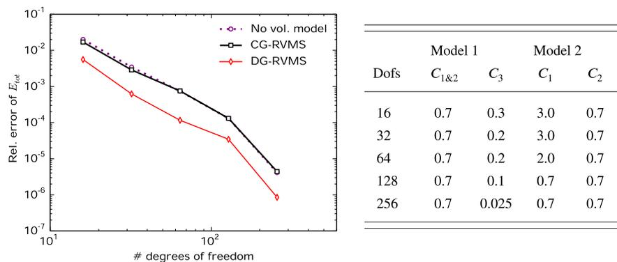
**FIGURE 9** Energy convergence with uniform mesh refinement at  $t = 8\pi$  for basis functions of  $p = 3$ . CG-RVMS, continuous Galerkin residual-based variational multiscale; DG-RVMS, discontinuous Galerkin residual-based variational multiscale; Dofs, degrees of freedom [Colour figure can be viewed at [wileyonlinelibrary.com](http://wileyonlinelibrary.com)]
