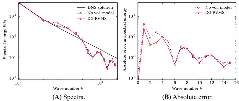
**FIGURE 12** Spectral energy obtained with four discontinuous Galerkin elements of  $p = 3$  and 16 degrees of freedom. A, Spectra; B, Absolute error. DG-RVMS, discontinuous Galerkin residual-based variational multiscale; DNS, direct numerical simulation [Colour figure can be viewed at [wileyonlinelibrary.com](http://wileyonlinelibrary.com)]
