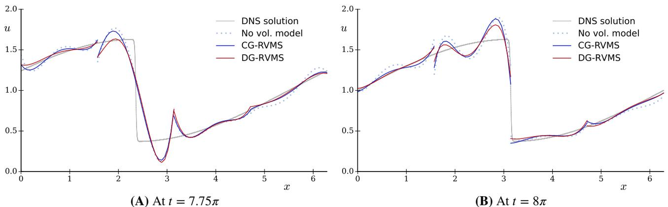
**FIGURE 7** Example solutions with and without the proposed discontinuous Galerkin residual-based variational multiscale (DG-RVMS) model, using four discontinuous Galerkin elements of  $p = 4$ . A, At  $t = 7.75\pi$ ; B, At  $t = 8\pi$ . CG-RVMS, continuous Galerkin residual-based variational multiscale; DNS, direct numerical simulation [Colour figure can be viewed at [wileyonlinelibrary.com](http://wileyonlinelibrary.com)]
