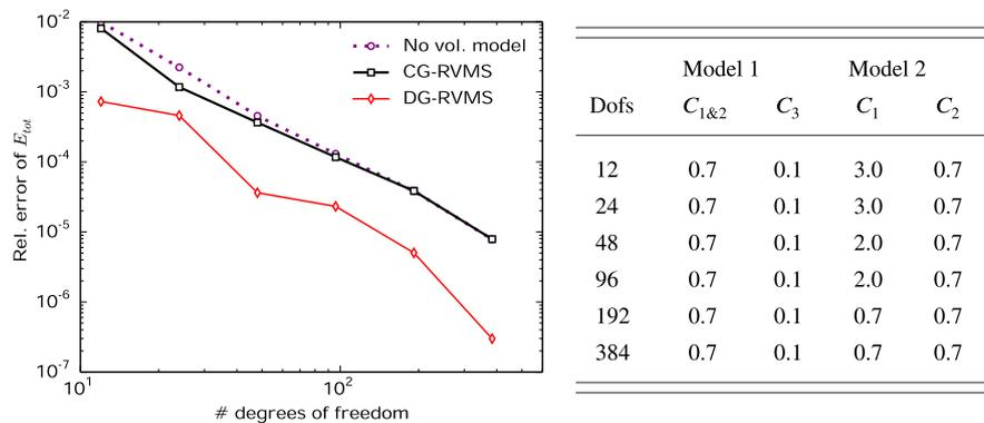
**FIGURE 8** Energy convergence with uniform mesh refinement at  $t = 8\pi$  for basis functions of  $p = 2$ . CG-RVMS, continuous Galerkin residual-based variational multiscale; DG-RVMS, discontinuous Galerkin residual-based variational multiscale; Dofs, degrees of freedom [Colour figure can be viewed at [wileyonlinelibrary.com](http://wileyonlinelibrary.com)]
