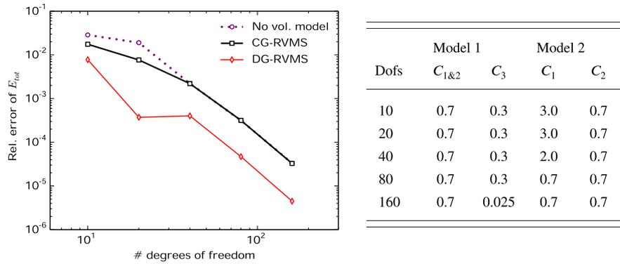
**FIGURE 10** Energy convergence with uniform mesh refinement at  $t = 8\pi$  for basis functions of  $p = 4$ . CG-RVMS, continuous Galerkin residual-based variational multiscale; DG-RVMS, discontinuous Galerkin residual-based variational multiscale; Dofs, degrees of freedom [Colour figure can be viewed at [wileyonlinelibrary.com](http://wileyonlinelibrary.com)]
