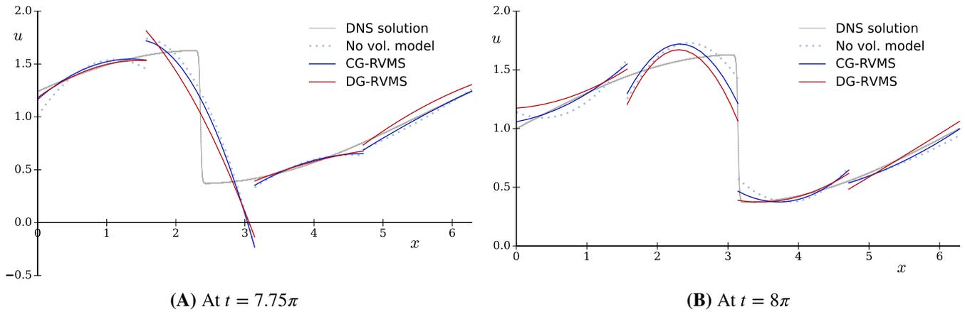
**FIGURE 5** Example solutions with and without the proposed discontinuous Galerkin residual-based variational multiscale (DG-RVMS) model, using four discontinuous Galerkin elements of  $p = 2$ . A, At  $t = 7.75\pi$ ; B, At  $t = 8\pi$ . CG-RVMS, continuous Galerkin residual-based variational multiscale; DNS, direct numerical simulation [Colour figure can be viewed at [wileyonlinelibrary.com](http://wileyonlinelibrary.com)]
