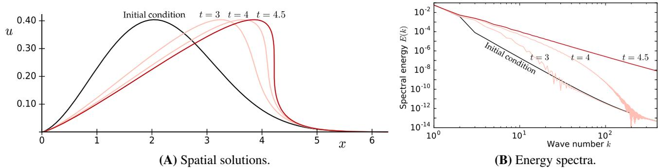
**FIGURE 2** Solution of the nonlinear transport equation at different time instants. A, Spatial solutions; B, Energy spectra [Colour figure can be viewed at [wileyonlinelibrary.com](http://wileyonlinelibrary.com)]
