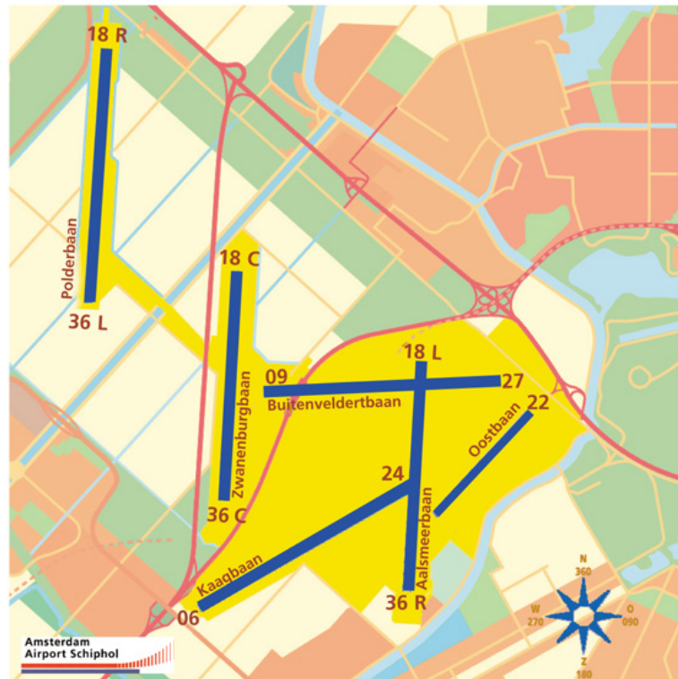
Figure 4.3: Runways of Schiphol, given with name and code to specify direction it is used in [1]
