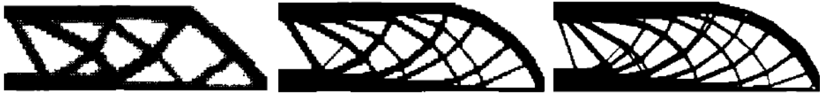
Figure 2.2: Mesh refinement dependency for the optimal topology. Solutions for a discretization with: 1350, 2400 and 8600 elements [6]
