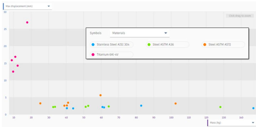
Figure 2.5: Plots from an explorative study done by Buonamici et al. in the Autodesk Fusion 360 Generative Design tool [3]
