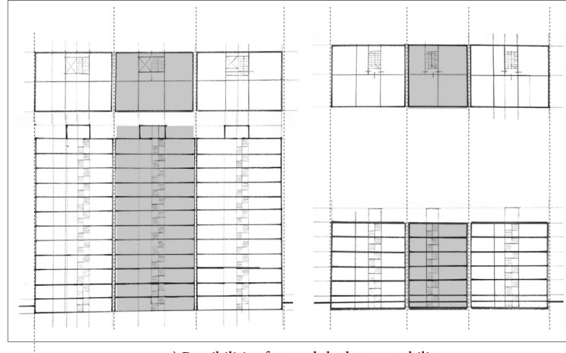
c) Possibilities for module demountability.
