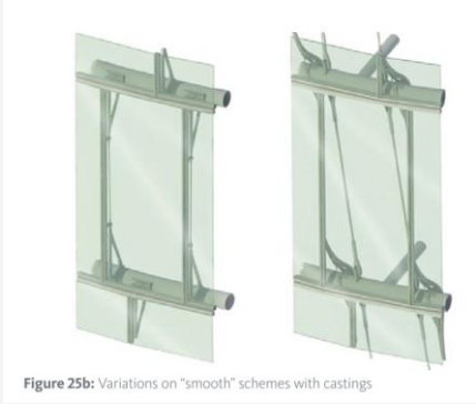
Figure 25b: Variations on "smooth" schemes with castings
