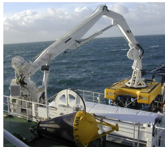
(b) Articulated cranes are present on almost any ship for cargo transfer in port [66].
