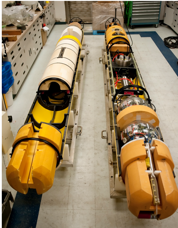
Figure 5.1: This photo of the insides of a 6000m-capable seafloor imaging AUV shows the space required for buoyancy material and pressure hulls [15]
