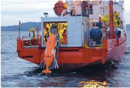
(a) A custom launch and recovery system [38].
