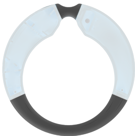
Figure 16. The links (in black) fulfil both a structural and a functional purpose for the MedRing and are considered “available space” for the integration of the miTAS.
