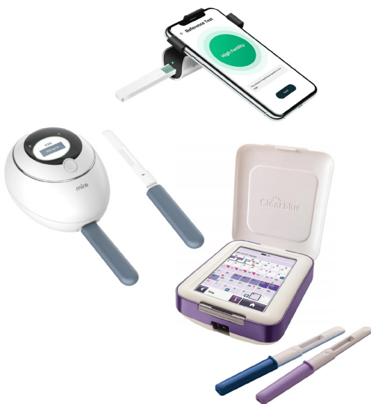
Figure 7. Despite looking similar to OPK's, all the HMS displayed here incorporate biosensors to yield results.
