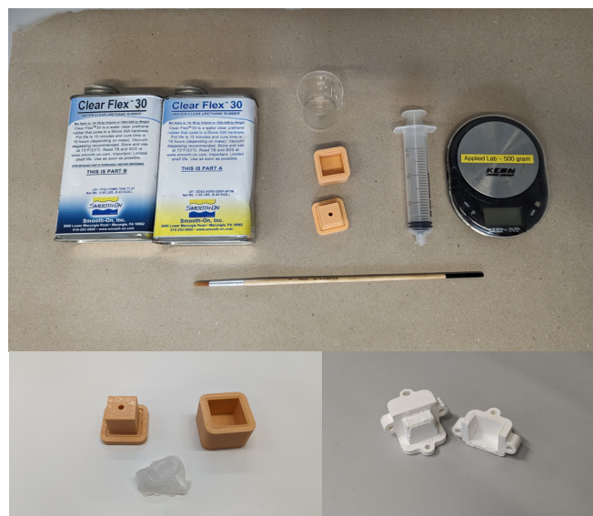
Figure 25. Top: tools and materials used for casting the membrane. Bottom left: first attempt. Bottom right: last attempt
