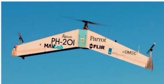
Figure 1. The DelftaCopter tailsitter UAV in hovering flight. DelftaCopter has a single large rotor with collective and cyclic blade pitch control, two small torque countering tip propellers and a pair of delta-wings placed in biplane configuration. The tips form the landing legs and provide yaw stability in forward flight. It weighs 4.3 kg and was designed to fly 60 km in the Outback Medical Challenge 2016. 15
