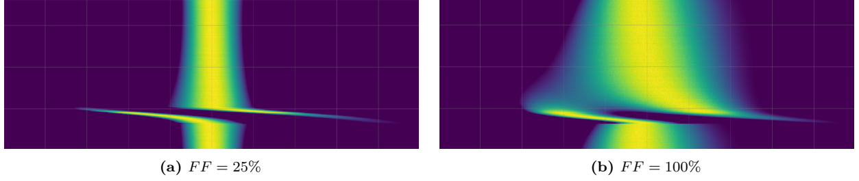
Figure 4.6: Example of data visualization after processing for V_{total} = 10 kV, r_2 = 0.625 and \dot{B} = 2.8 T/s
