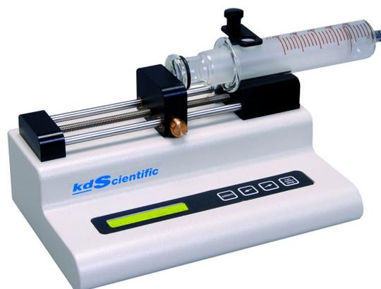
Figure 3.2: The syringe pump used to provide the sorbent flow rate
