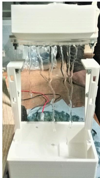
Figure 2.13: Inhomogeneous sorbent flow (acrylic test) [13]
