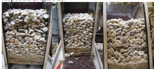
Figure 2 Gravel after application of the Biogrout process for five (left and middle) and nine (right) flushes. The box in the middle also contained 7% sand.
