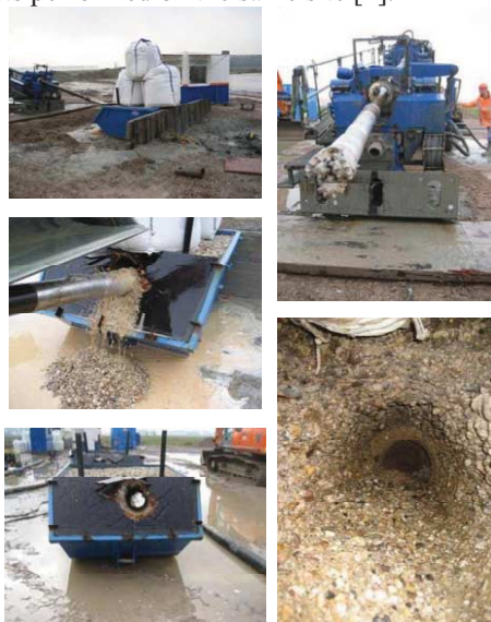
Figure 3 Drilling tests in a 3 m 3 cemented gravel container.
